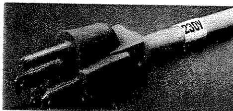
Figure 2-1. Instrument Configured for 198 to 252 Vac Operation
