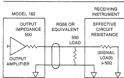
**Figure 3-2. Signal Termination**
