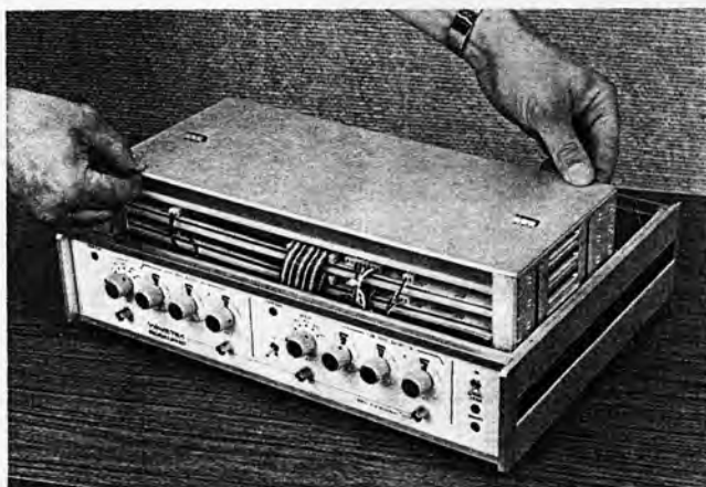
Figure 5-3. Moving Card Cage Out of Instrument
