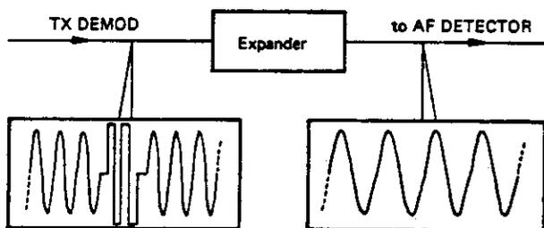
AF signal with burst signaling (between marking lines) before the expander and without signaling after the expander.
