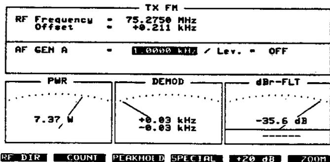
Weighted S/N ratio: The display on the dBr meter shows that the device under test in this case exhibits a weighted S/N ratio of -35.6 dB (CCITT weighting).
