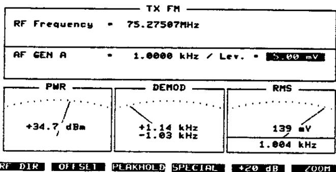
**Carrier frequency:** As soon as the *COUNT* function is called up, the *RF Frequency* field indicates the carrier frequency of the device under test
