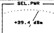
Selective power measurement: Here the SEL.PWR meter shows the measured value with dBm units because these units were declared in the *RF Power* field of the GENERAL PARAMETERS mask.
