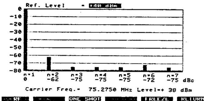
Harmonics: The harmonics measurement shows an absolute level of +38 dBm for the fundamental (75.2750 MHz), a relative level of -62 dBc for the second harmonic, -75 dBc for the third harmonic, etc. With 4 μW (+38 dBm - 62 dBc = -24 dBm) the second harmonic exceeds the permissible limit.
