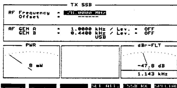
Spurious modulation: on the dBr meter you can read the noise voltage with CCITT weighting.
