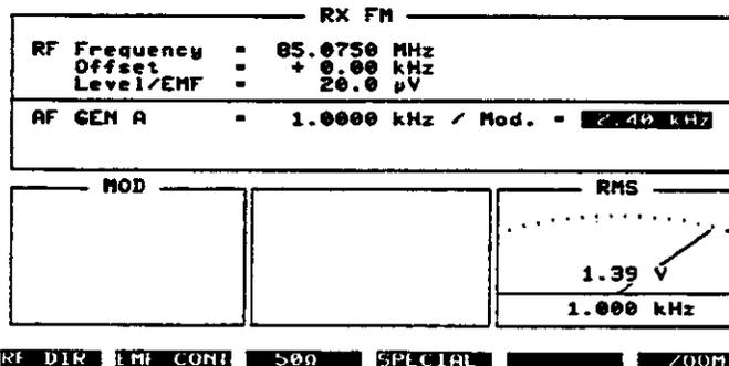
**Basic RX setting:** In the RX mask the following operating parameters are declared here: RF is the active RF socket, RF level = 20 μV/EMF, channel frequency = 85.075 MHz,  $f_{mod} = 1 \text{ kHz}$ , FM modulation, test modulation = 2.4 kHz.
