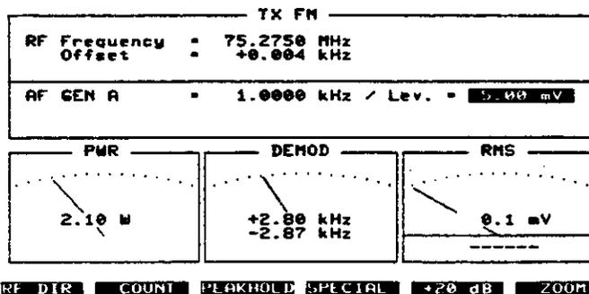
**Basic TX setting:** The following operating parameters are declared in the mask for example: channel frequency = 75.2750 MHz,  $f_{mod} = 1 \text{ kHz}$ , modulation = FM, RF socket is active input, *Lev* field is active and expects, depending on test to be performed, entry or variation of modulation level.
