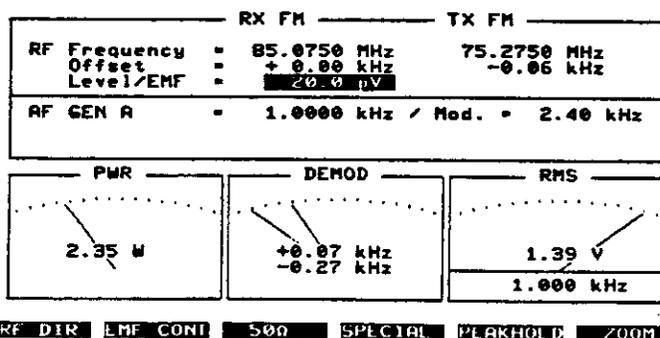
Basic DUPLEX setting: Here the following parameters are specified in the DUPLEX mask: RF is the active socket,  $f_{TX} = 85.075$  MHz,  $f_{RX} = 75.275$  MHz, RF level = 20  $\mu$ V,  $f_{mod} = 1$  kHz, FM modulation, test modulation = 2.4 kHz.
