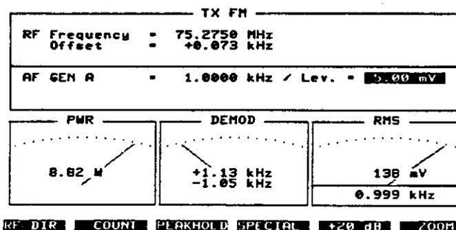
**Transmitting power:** The PWR meter, which is always displayed in the TX mask, shows the average carrier power of the device under test. The measurement is broadband, so the channel frequency (*RF Frequency* field) is insignificant.
