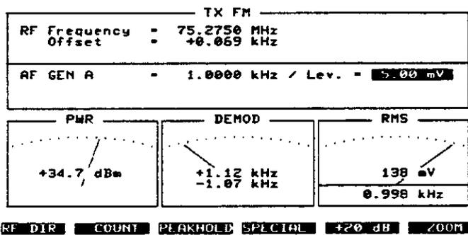
**Frequency offset:** The *Offset* display field indicates that the carrier frequency of the device under test deviates from the rated channel frequency
