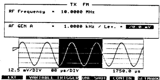
**Timing measurement:** First the shiftable edge of the timing field was moved to the negative amplitude of the signal curve with the handwheel. **<SETMARK>** defined this point as the new start position of the timing field, which can then be expanded as required. The portion of the signal marked here has a duration of 1750 μs.
