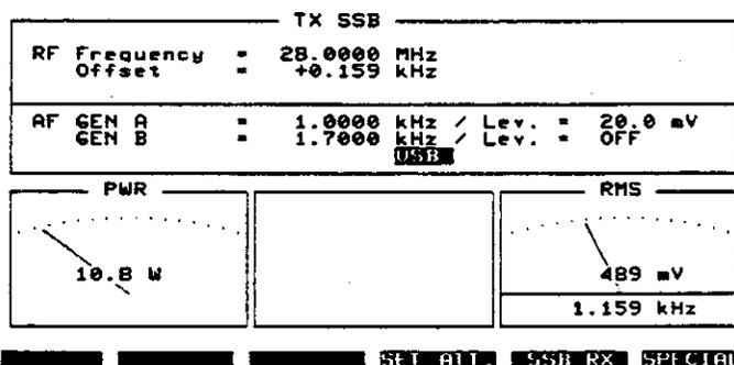
**Frequency offset:** in the Offset field you can read the difference between the measured RF frequency and the figure entered in the *RF Frequency* field.
