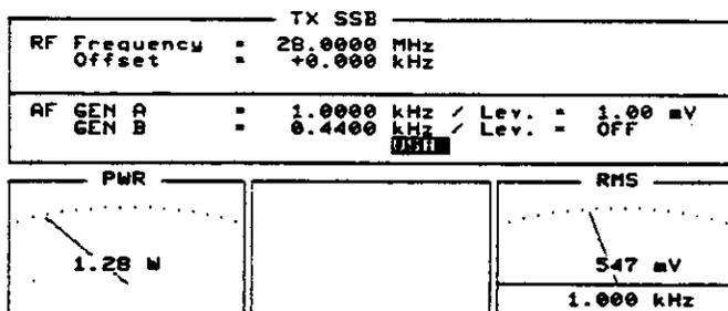
TX mask: the instrument is set for 28 MHz channel frequency, the upper sideband is selected and the modulation level of generator GEN A is 1 mV for a modulation frequency of  $f_{\text{mod}} = 1 \text{ kHz}$ .
