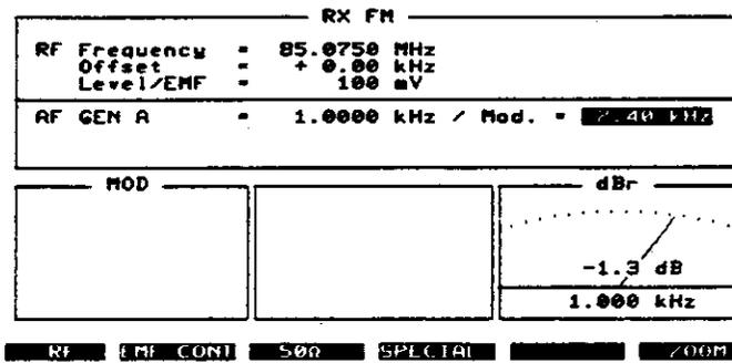
**Limiter characteristic:** After the AF level has been normalized at  $2 \mu\text{V}$  RF level by calling up the dB meter, the meter now shows -1.3 dB at 100 mV RF level.
