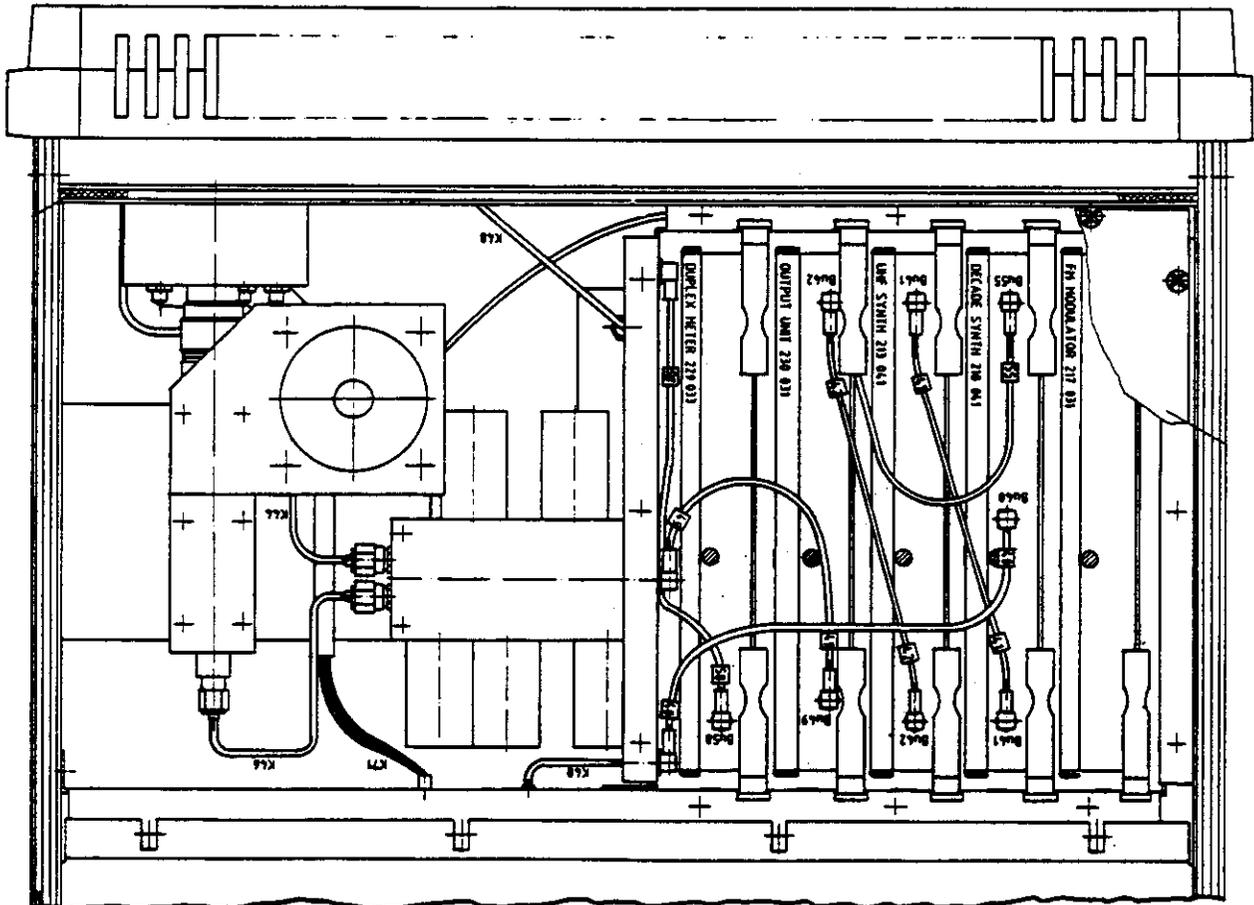
Partial view of chassis with bottom half of shell and cover plate removed. Cables 40 and 49 have to be undone to install the duplex stage.
