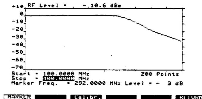
**Marker function:** The marking line, which is adjustable with the spinwheel, permits exact measurement of relative level. The *Marker Freq.* field indicates the frequency at the current position of the marker, the *Level* field shows the corresponding relative level.
