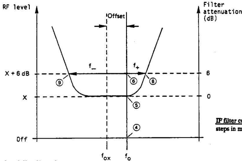
**IF filter curve:** The numbers refer to the different steps in manual measurement.
