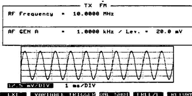
**AUTOTRIG mask:** Display of the GEN A modulation signal. The vertical deflection coefficient is 12.5 mV/div, the horizontal deflection coefficient is 1 ms/div.
