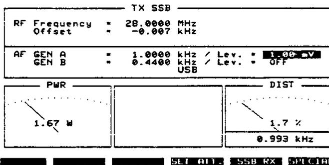
Distortion factor: the distortion factor of the test item can be read on the DIST meter.
