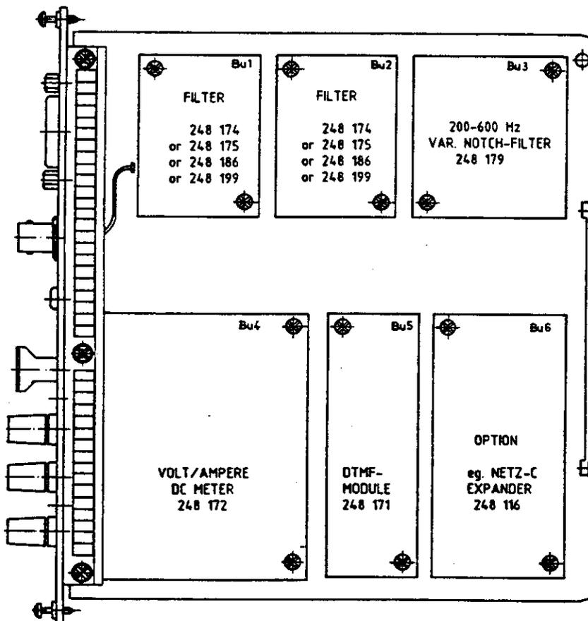
The various modules have locations on the OPTION CARD (figure). Only locations Bu 1, Bu 2 and Bu 6 offer a choice: Bu 1 and Bu 2 can each hold one of the four AF filters, Bu 6 can hold the C-Net expander or another special option. For making contact, each module has a plug connector that uniquely matches the corresponding socket connector on the OPTION CARD. Before installing the DC V/A meter, first remove the shield from the OPTION CARD that covers the leadthrough of the connecting sockets.
