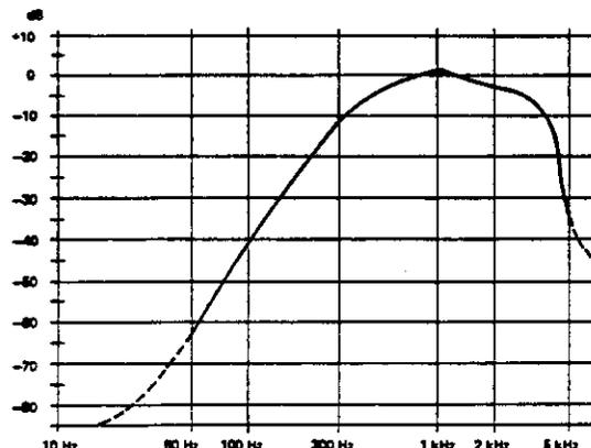
In receiver testing you can, if you wish, perform weighted measurements of level, SINAD and distortion. All you have to do is to tap the CCITT key in the AF field of the front panel. The yellow LED will then illuminate; the label *FLT* is added to the meter designations "RMS" or "dBr", "SINAD" and "DIST" to avoid any confusion with unweighted measurement. Tapping the CCITT key once more cuts the filter out of the signal path.
