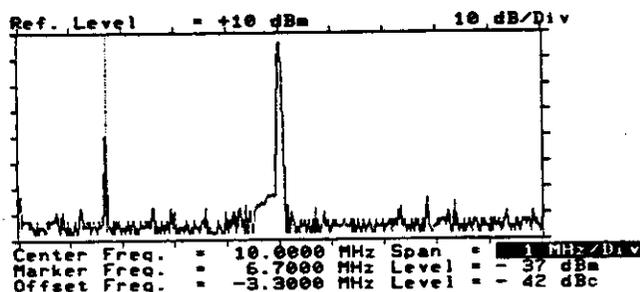
**Marker submask:** The marker (vertical dotted line) has been set with the handwheel to 6.7 MHz. The level of the corresponding spectral component reaches -37 dBm. The marker is offset from the centre frequency (10 MHz) by -3.3 MHz; the level measured at the marker frequency is -42 dBc below the level at centre frequency.
