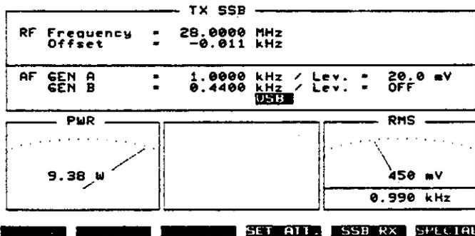
RF power: the PWR meter shows the average carrier power of the radio set. Measurement is broadband, so the channel frequency (*RF Frequency* field) is unimportant.
