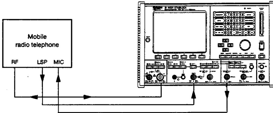
Cable connections: 4031 (MOD GEN) ---> microphone input MIC of mobile; for measuring the modulation characteristics of the mobile transmitter. AF output (LSP) of mobile ---> 4031 (VOLTM); for measuring the sensitivity and demodulation characteristics of the mobile receiver. RF <---> RF = RF signal path.
