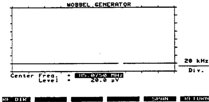
**SWEEP GENERATOR:** When the monitor shows this mask, the output signal of the 4031 signal generator is swept, here for example with 200 kHz sweep width (20 kHz/div x 10 div). Parallel to the sweep process a marker (space) moves on the frequency axis that appears at the bottom of the window, the position of which indicates the current signal frequency.
