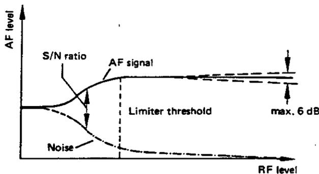
**Limiter characteristic:** The AF output level of the radio set is virtually independent of the RF input level after the limiter has responded.
