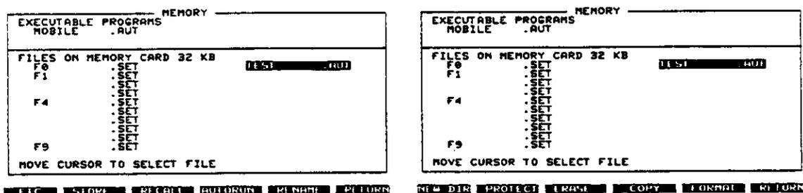
The two pages of the **MEMORY** mask: The first page (left) is only different from the second page in its softkey functions. Here, for example, the so-called cursor bar marks the entry **TEST.AUT** in the directory **FILES ON MEMORY CARD**.
