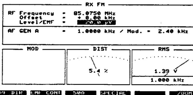
Demodulation distortion: The DIST meter shows a distortion factor of 5.4 % for the device under test.
