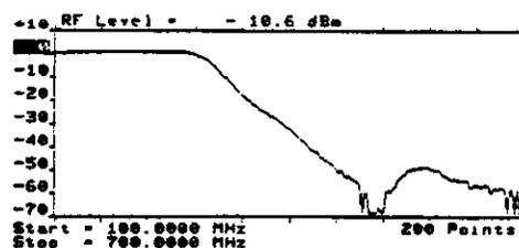
Lowpass-filter curves plotted with the tracking function: when analyzing passive networks it is always best to do without the unnecessary display dynamic range between 0 and +40 dB and instead to spread the useful dynamic range to between 0 and -70 dB. Then the curve becomes visible in the lower level range.
