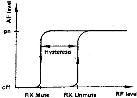
Squelch characteristic: When the increasing RF level on the antenna input of the radio set reaches the enabling threshold (RX Unmute) of the squelch, the latter enables the AF signal. When the decreasing RF level reaches the blocking threshold (RX Mute), the AF signal is blocked or muted. The hysteresis prevents uncontrolled response of the squelch when the RF level alters minimally.
