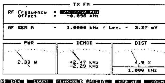
Modulation distortion: The DIST meter confirms that the modulation distortion of the device under test does not exceed the permissible limit value.
