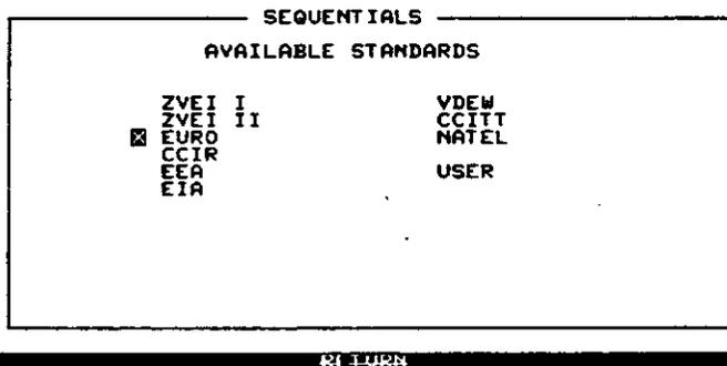
**SEQUENTIALS submask:** This submask of the basic sequential mask permits you to select the tone sequence whose parameters are to be valid for the encoder and decoder. In this case the *EURO* tone sequence has been selected.
