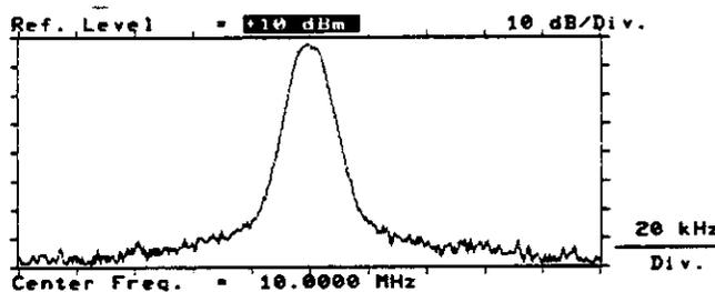
**Basic analyzer mask:** A reference level of +10 dBm is set in the Ref. Level scroll field. The dynamic range of the analyzer display is thus matched optimally to the dynamic range of the applied 10-MHz signal.
