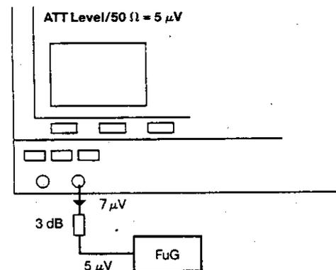
If you work with external pre-attenuation, and this is correctly entered in the *Pre-attenuation* field, you do not have to make any further allowance for the pre-attenuation.
