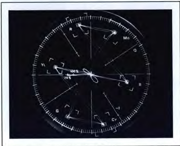
Fig 1—Vector display—full field color bars, 75% amplitude, 100% white reference, 10% set-up. Conforms to EIA standard RS189. Type 141 NTSC Test Signal Generator used as a signal source.
