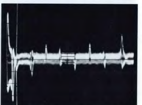
Fig 12: Modulated staircase signal viewed on a Type 520 Vectorscope in the differential phase mode. Photo indicates combined differential phase of both instruments.
