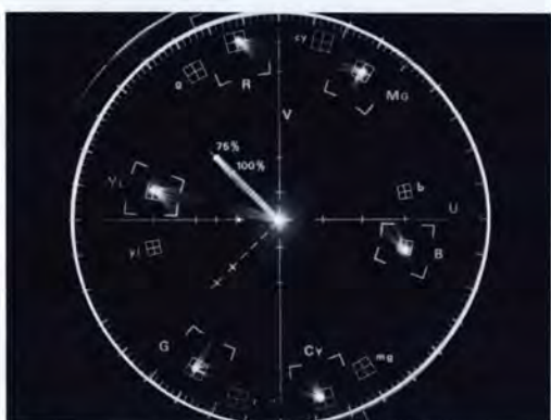
Fig. 1B—Vector NTSC presentation of PAL color bar signal.
