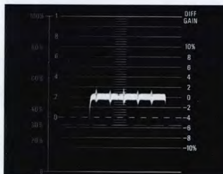
Combined differential gain of Type 520 PAL Vectorscope and Type 141 Generator. Minor scale divisions equal \frac{1}{2}\% differential gain.
