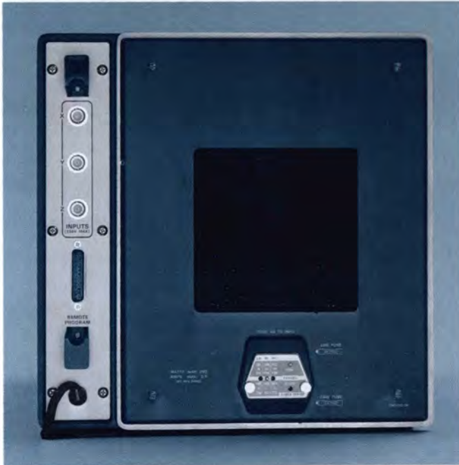
Rear panel of Type 611 Storage Display Unit.
