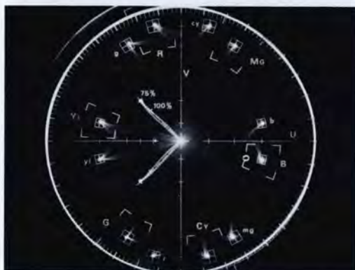
Fig. 1A—Vector PAL presentation of PAL color bar signal.
