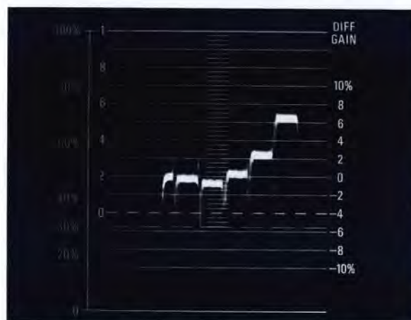
Fig 2—Type 520 PAL and Type 141 system being used to measure differential gain of a typical cascade of video amplifiers. Indicated differential gain is 6\frac{1}{2}\% .
