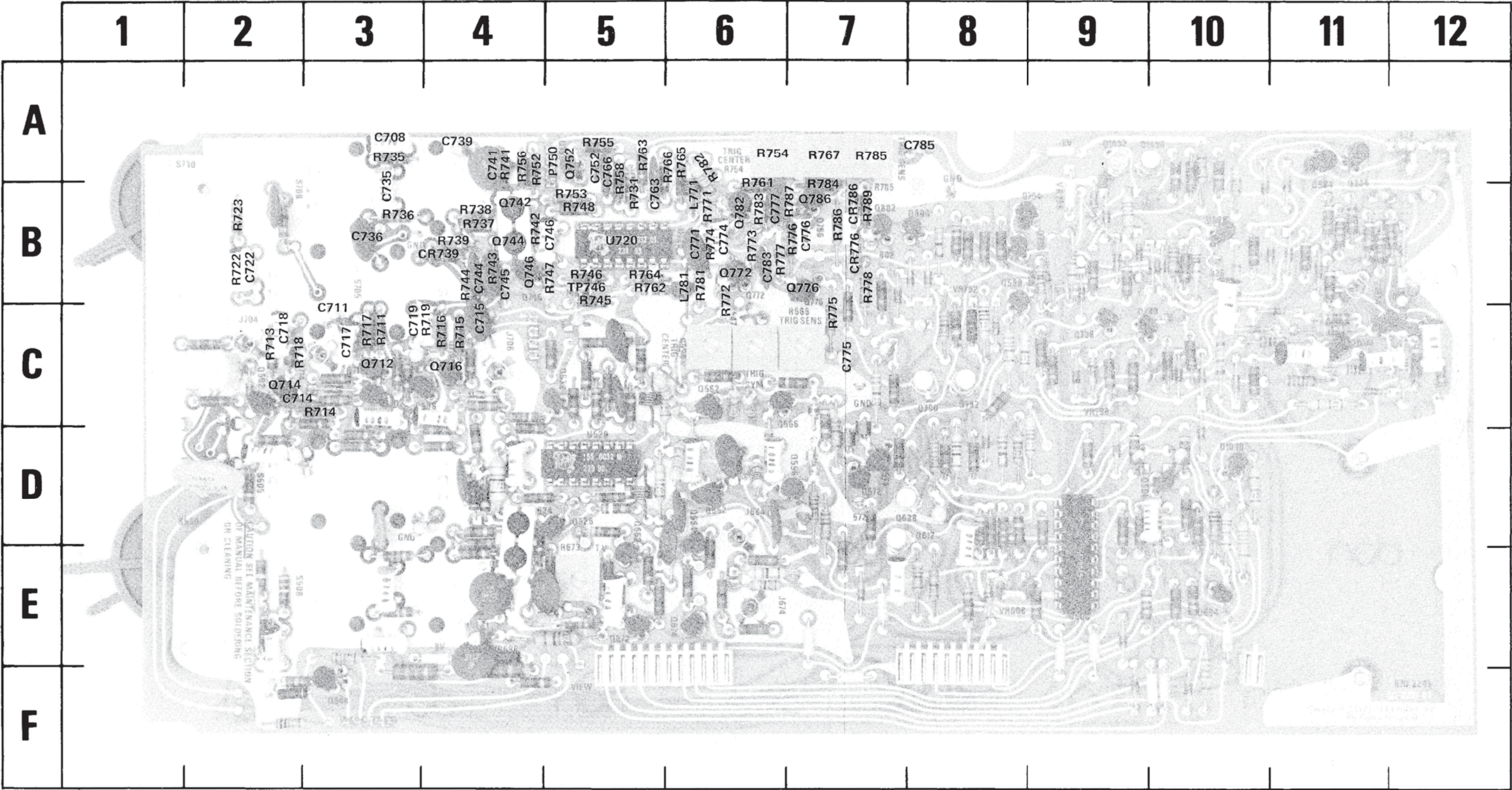
Fig. 7-13. P/O A8 Trigger Generator And Sweep Logic circuit board.
