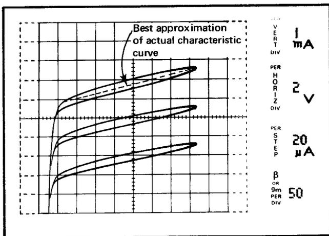
Fig. 2-23. Example of a display exhibiting looping.
