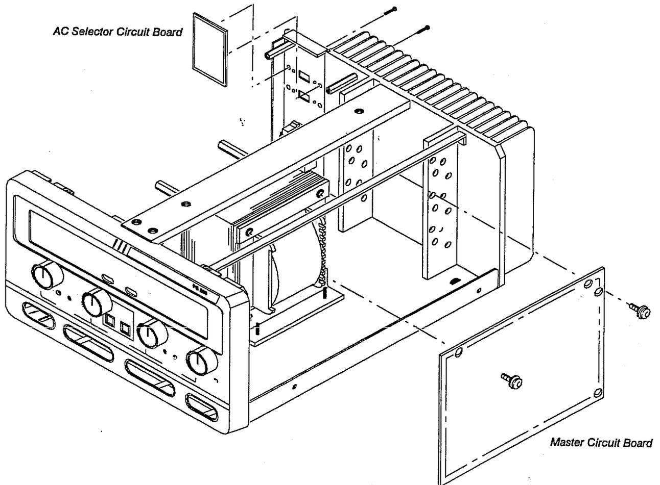
Figure 6-3: AC Selector and Master Circuit Board Removal
