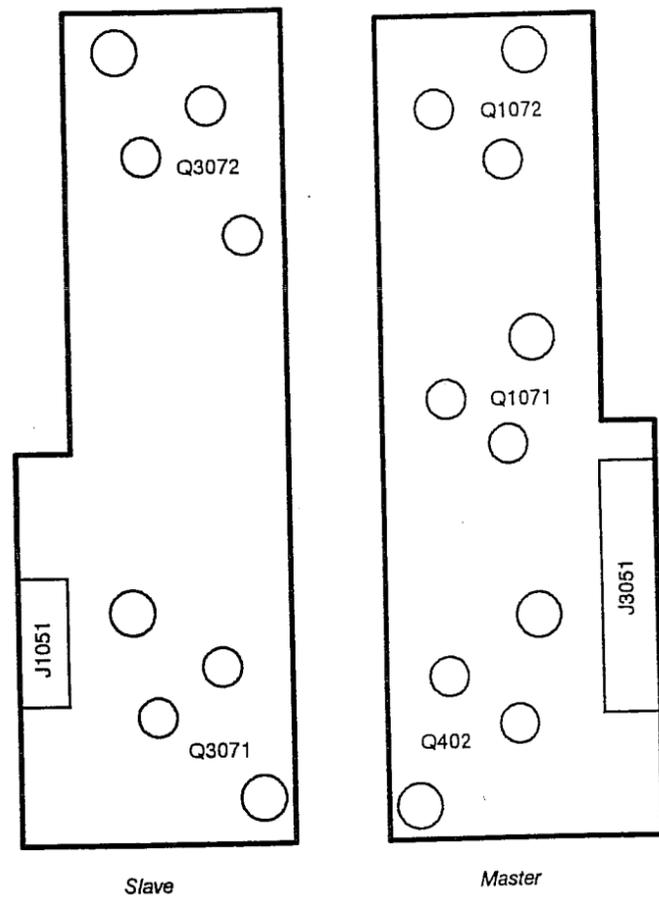
Figure 9-6: Power Transistors Circuit Boards
