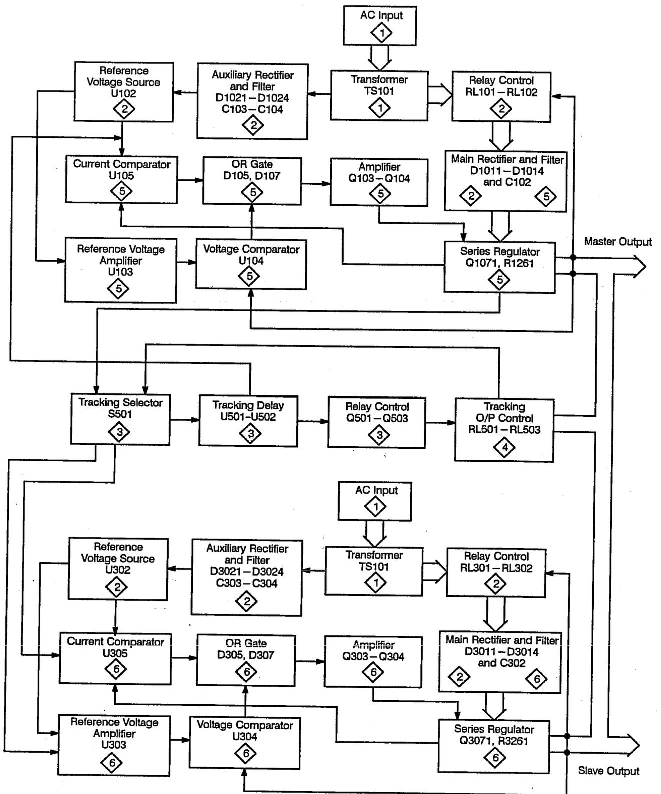
Figure 3-1: PS280 or PS283 Variable Outputs Block Diagram
