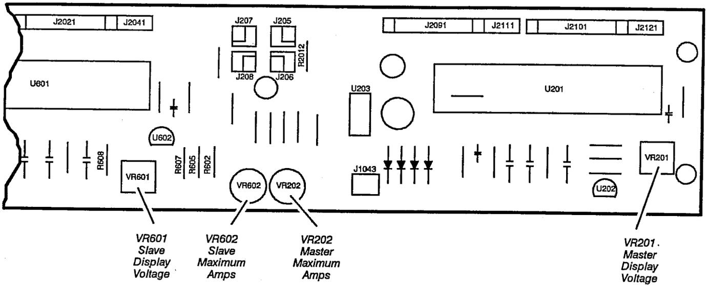
Figure 5-2: Display Assembly Circuit Board Adjustment Locations
