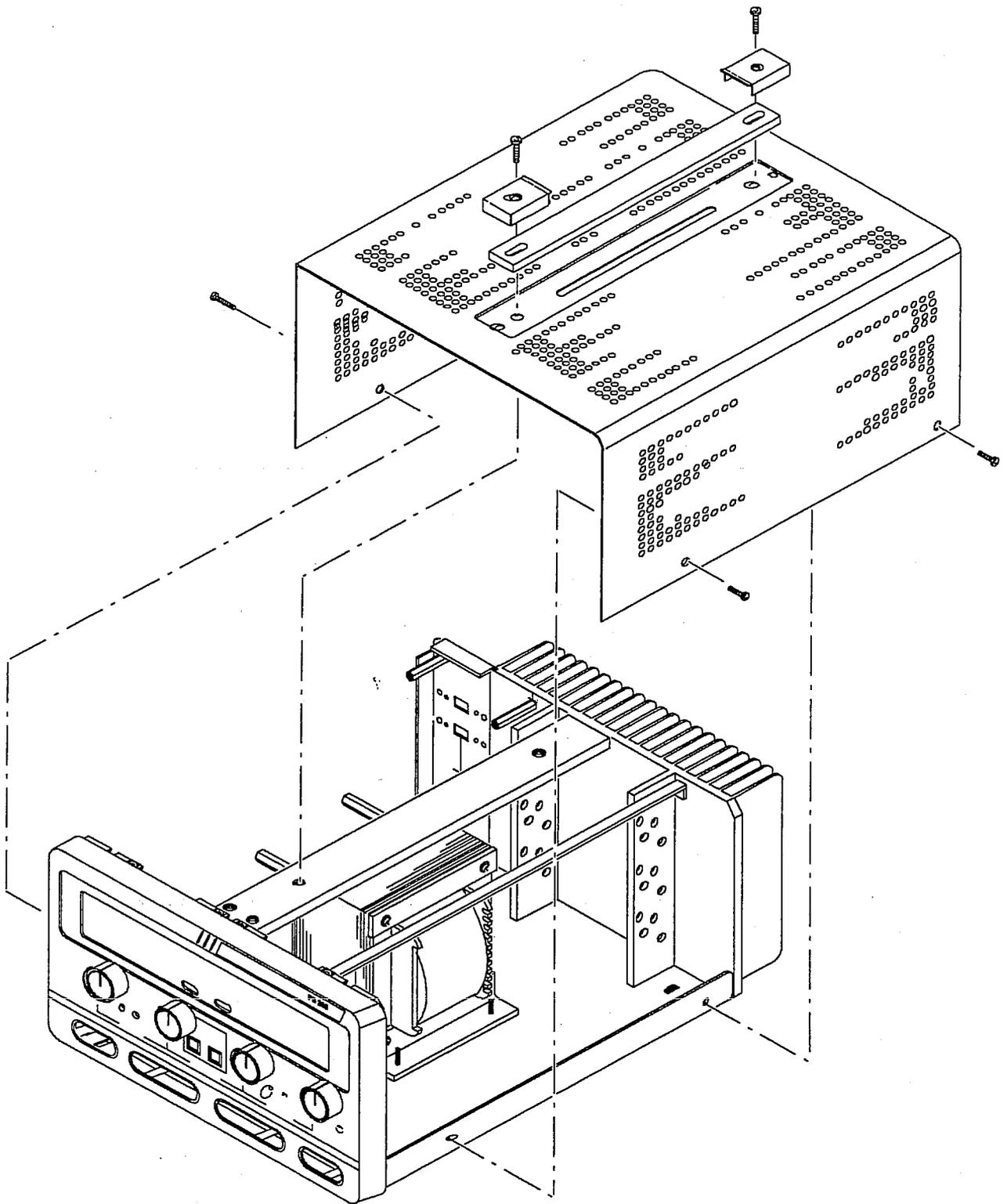
Figure 6-1: Top Cover Removal
