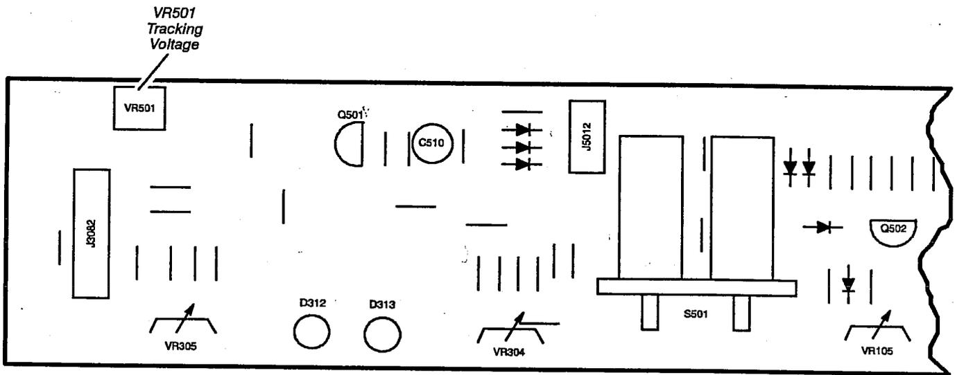
Figure 5-3: Front Panel Controls Circuit Board Adjustment Locations
