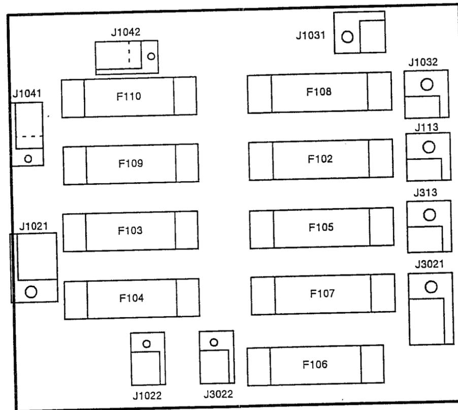
Figure 9-7: Fuse Circuit Board
