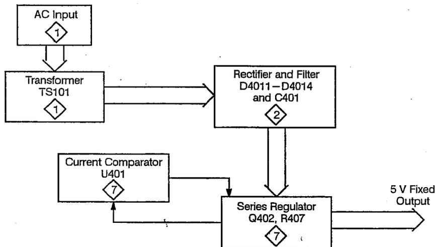
Figure 3-2: PS280 or PS283 5 V Block Diagram
