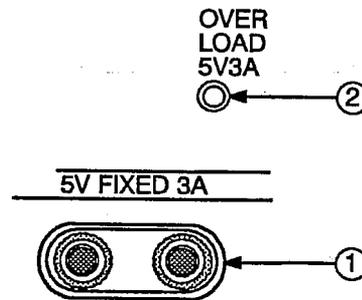
Figure 2-3: Fixed Power Supply Controls
