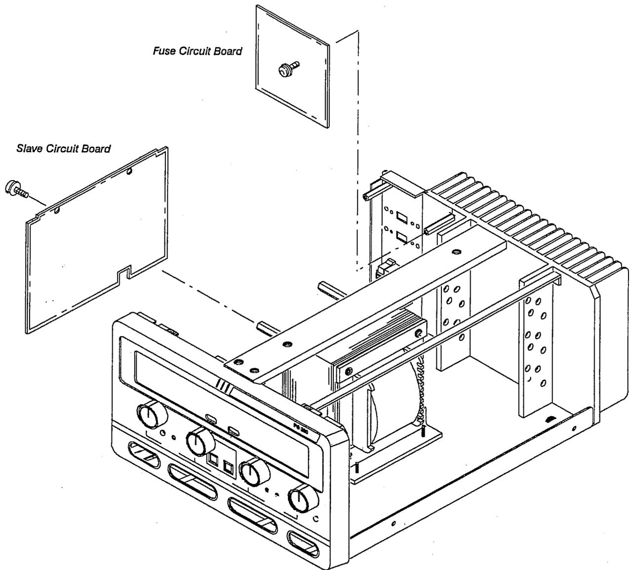
Figure 6-2: Slave and Fuse Circuit Board Removal
