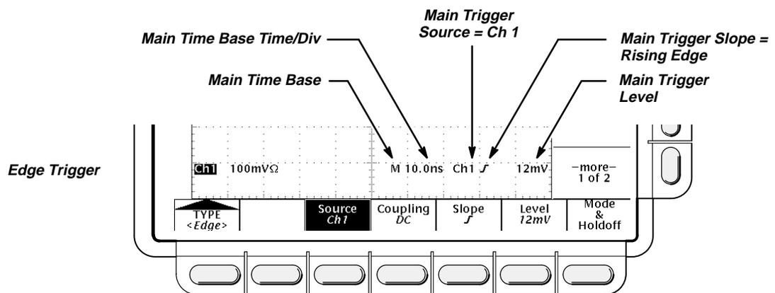
**Figure 3-60: Example Trigger Readouts**
