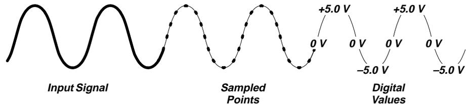
**Figure 2-4: Acquisition: Input Analog Signal, Sample, and Digitize**
