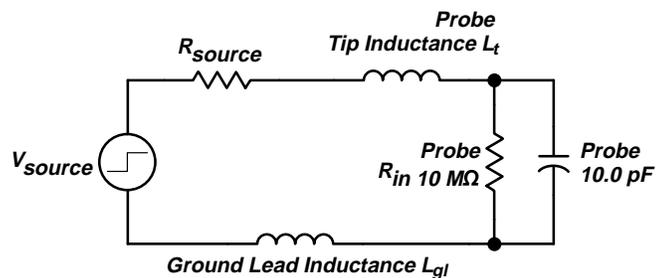
**Figure 3-35: A Probe Adds Resistance, Capacitance, and Inductance**
