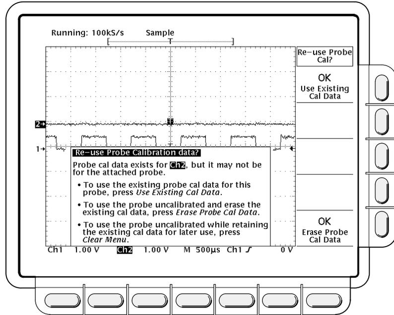
**Figure 3-40: Re-use Probe Calibration Data Menu**
