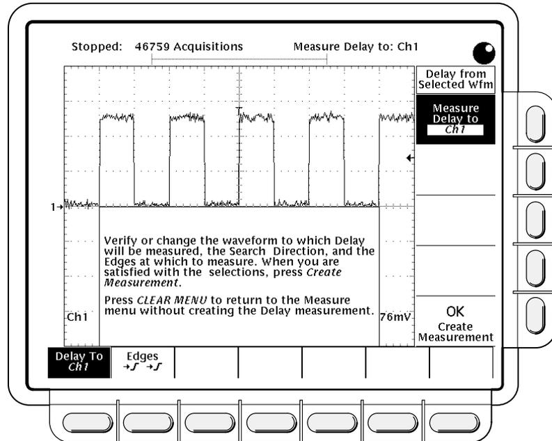
Figure 3-33: Measure Delay Menu—Delay To
