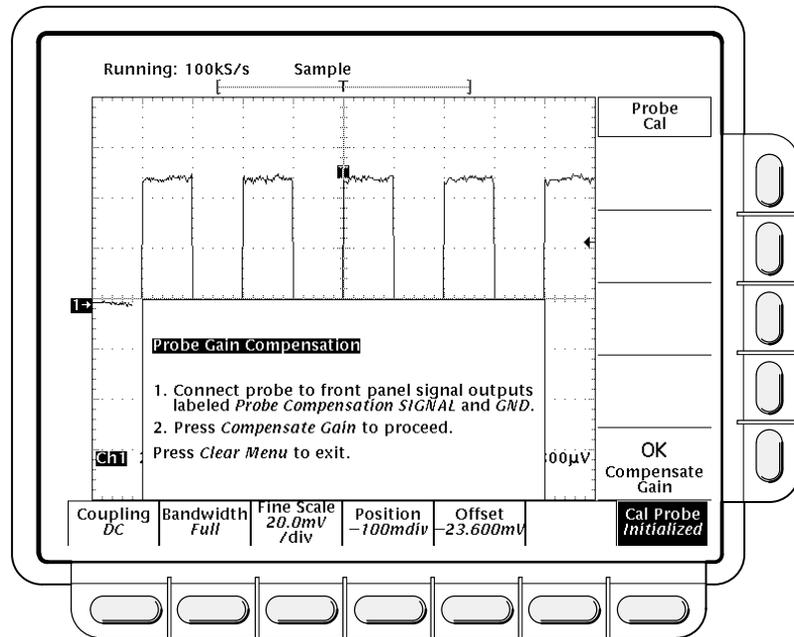
**Figure 3-39: Probe Cal Menu and Gain Compensation Display**
