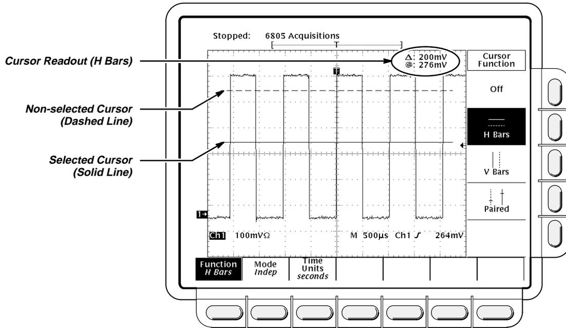
**Figure 3-6: H Bars Cursor Menu and Readouts**
