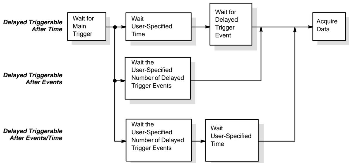
**Figure 3-9: Delayed Triggerable**
