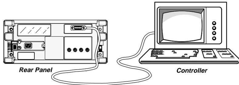
**Figure 3-50: Connecting the Digitizing Oscilloscope to a Controller**
