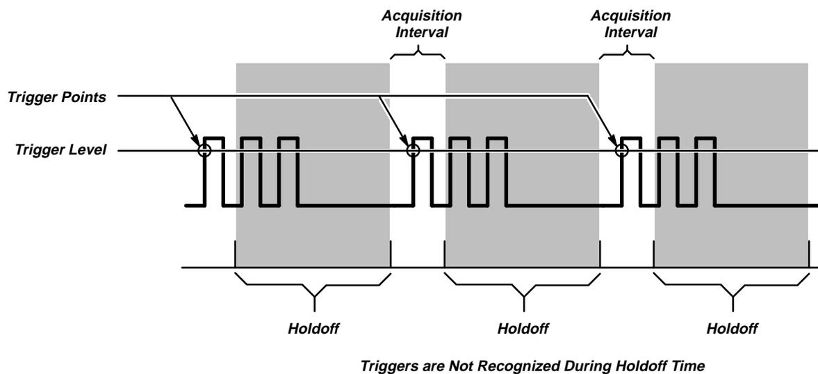
**Figure 2-2: Trigger Holdoff Time Ensures Valid Triggering**
