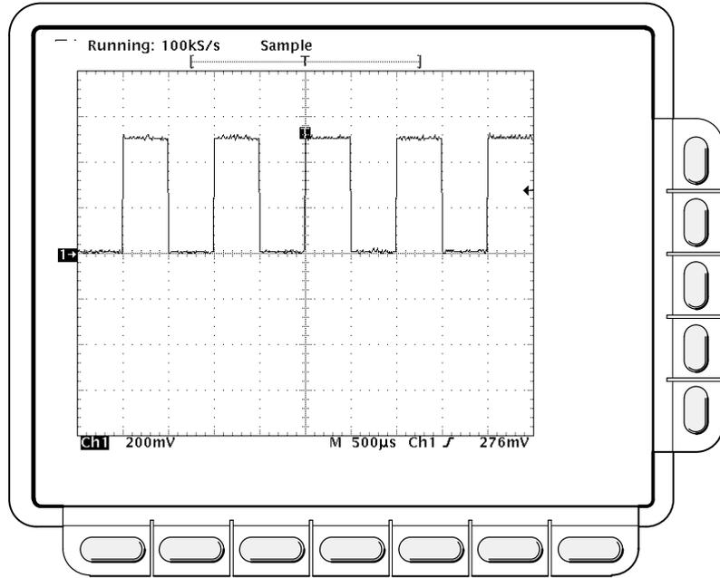
Figure 1-9: The Display After Pressing Autoset
