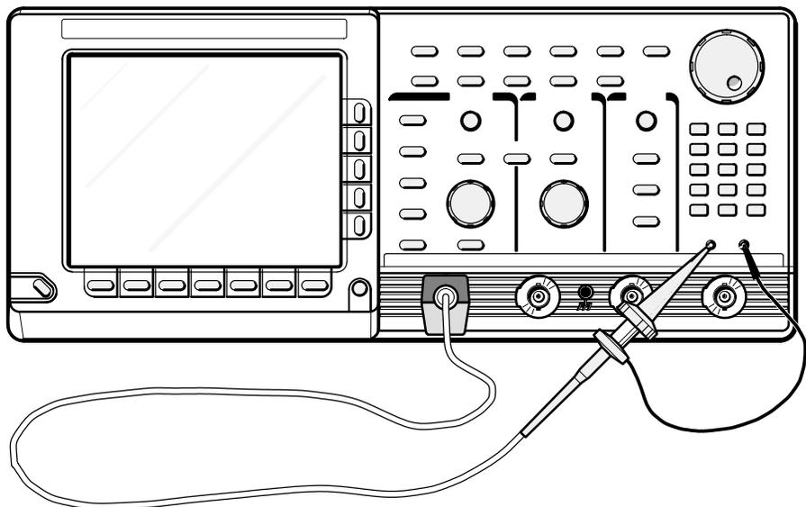
Figure 1-1: Connecting a Probe for the Examples
