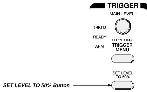
**Figure 1-4: Trigger Controls**
