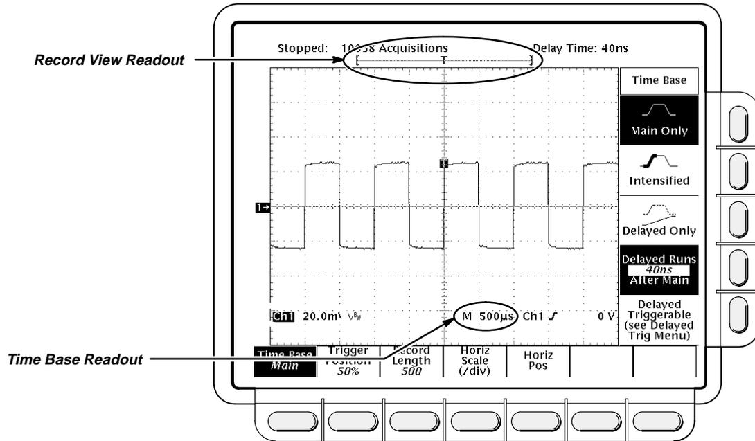
Figure 3-24: Record View and Time Base Readouts
