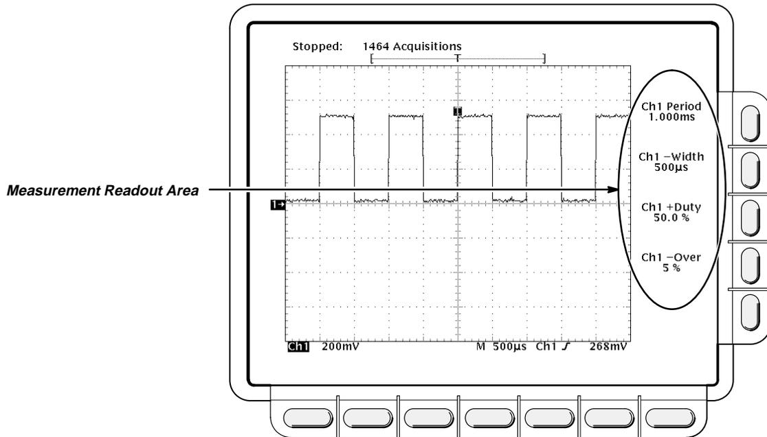
Figure 3-29: Measurement Readouts
