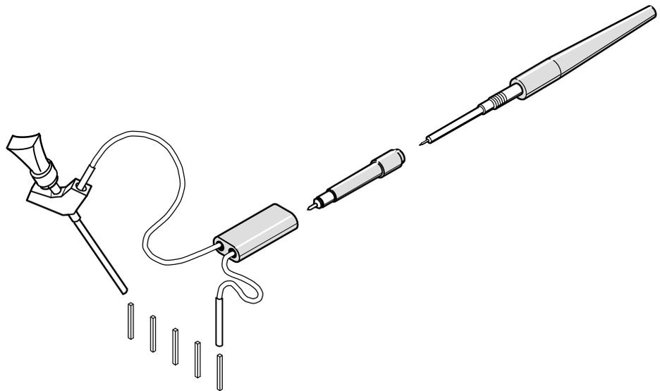
**Figure 3-38: Dual-Lead Adapter**
