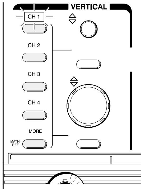
**Figure 1-11: The Channel Buttons and Lights (TDS 540 Shown)**
