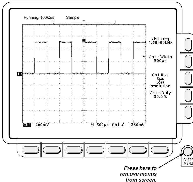
Figure 1-15: Four Simultaneous Measurement Readouts
