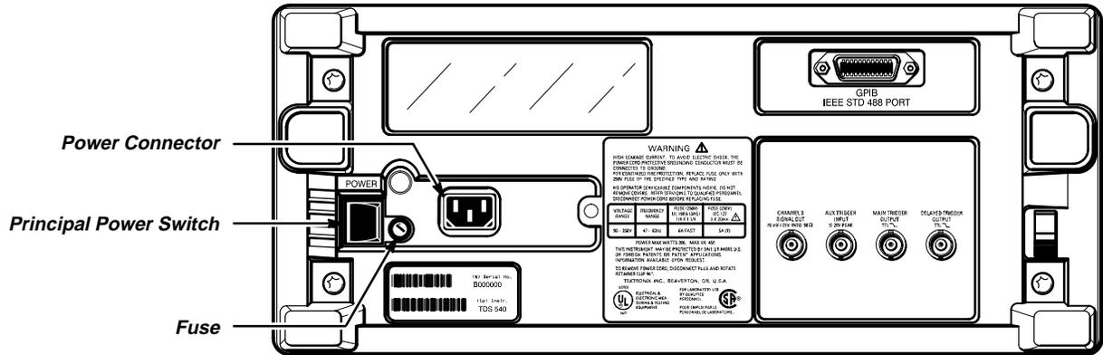
Figure i: Rear Panel Controls Used in Start Up
