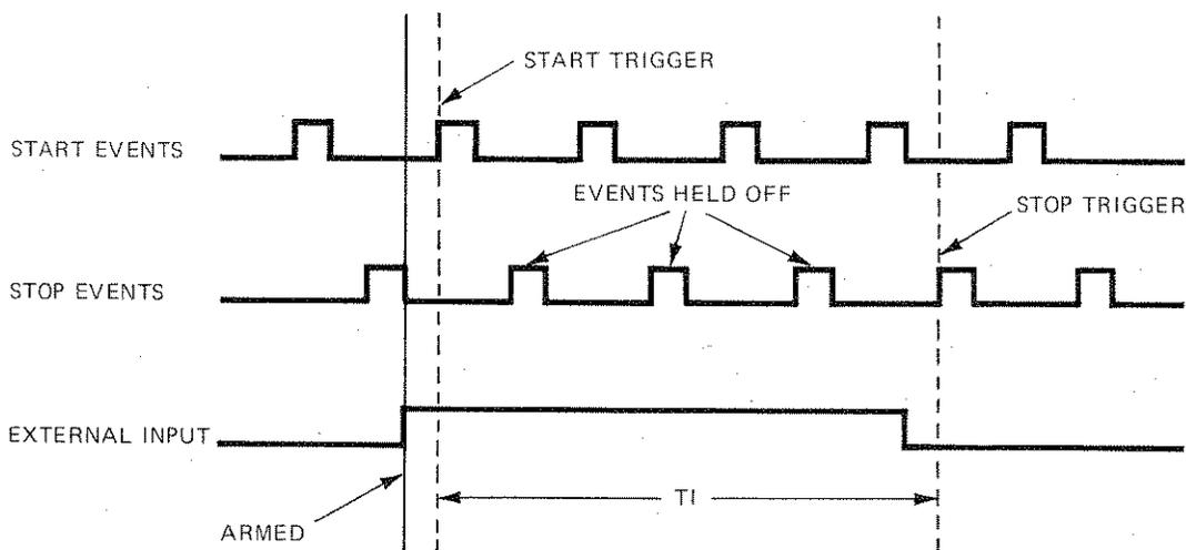
The number of events held off are counted and stored by the 5370A and can be displayed by pressing the DSP EVTS switch on the front panel.
