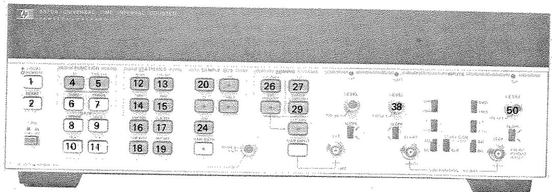
15. Press STD DEV13 and  $\pm$ T.I. switch27. Display should read less than 100 ps (this reading is the instrument's jitter). Notice that SAMPLE SIZE automatically goes to 100. For STD DEV measurements, SAMPLE SIZE must be  $\geq 100$ . Press MIN switch14 and minimum T.I. should be displayed. Press MAX switch15 and the maximum T.I. should be displayed. Press  $\pm$ T.I. ONLY26.
