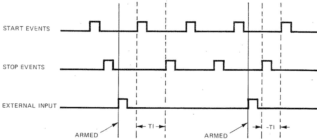
3-20. **EXTERNAL ARM/EXTERNAL HOLDOFF.** To operate the counter in the EXTERNAL HOLD-OFF mode, press the EXT HOLDOFF switch on the front panel. The selected trigger edge at the external input then arms the counter. The next START input pulse begins the measurement. The STOP pulses are held off as long as the external input holdoff is present as illustrated in the diagram.
