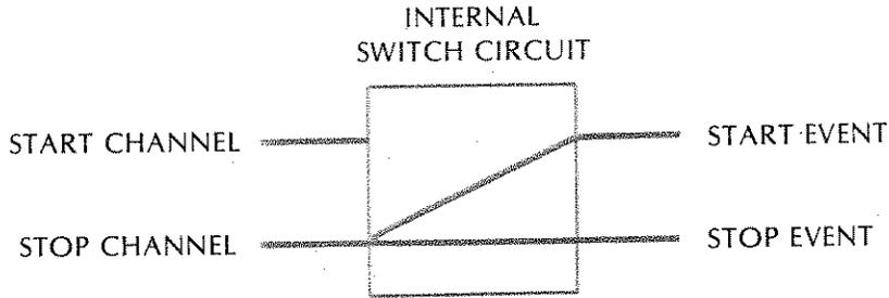
IN3 Input selection for operator convenience in switching input to different channels. START event = START channel input, STOP event = START channel input.
