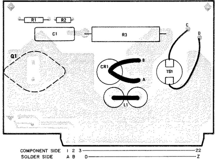
Figure 7-5. Output Diode Board (A4) Component Location
