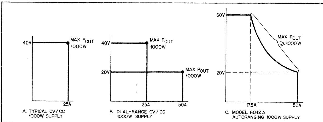
Figure 4-1. Output Characteristics; Typical, Dual-Range, and Autoranging Supplies
