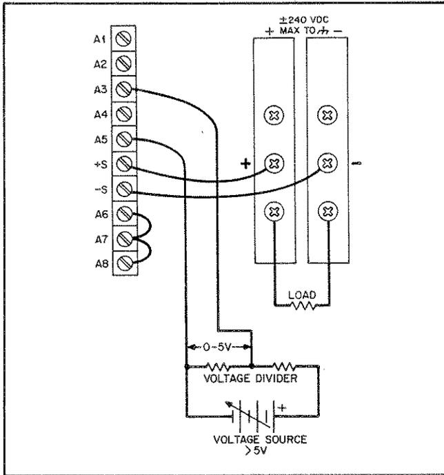
**Figure 3-12. Scaled Voltage Programming of Output Current**
