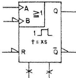
A positive-going transition at A or a negative-going transition at B triggers the one-shot. External timing components connect to non-logic inputs.
