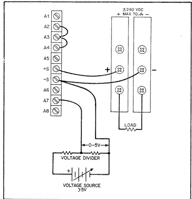
Figure 3-8. Scaled Voltage Programming of Output Voltage
