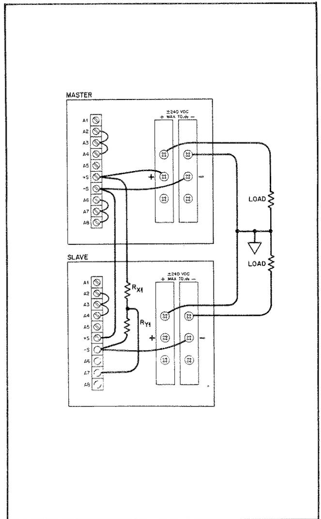
**Figure 3-16. Auto-Series Operation, Positive and Negative Outputs**
