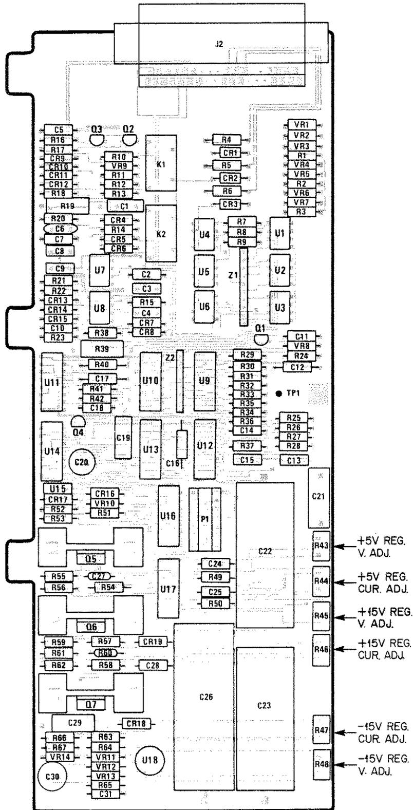
Figure A-14. Option 002 Board Component Location
