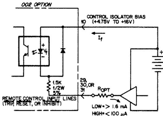
On state (logic low); Minimum forward current required ( $I_f$ ): 1.6 mA
