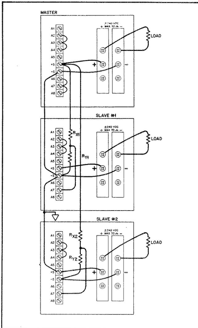
Figure 3-18. Auto-Tracking Operation, Positive and Negative Outputs
