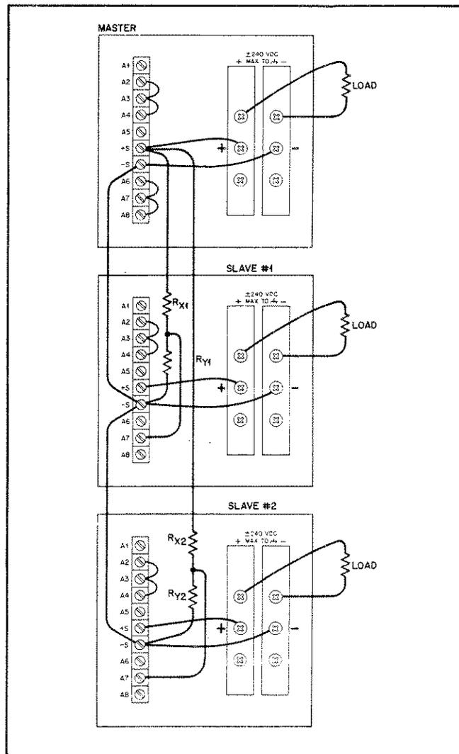
Figure 3-17. Auto-Tracking Operation
