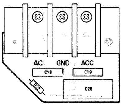
Figure 7-6. AC Filter Assembly Component Location
