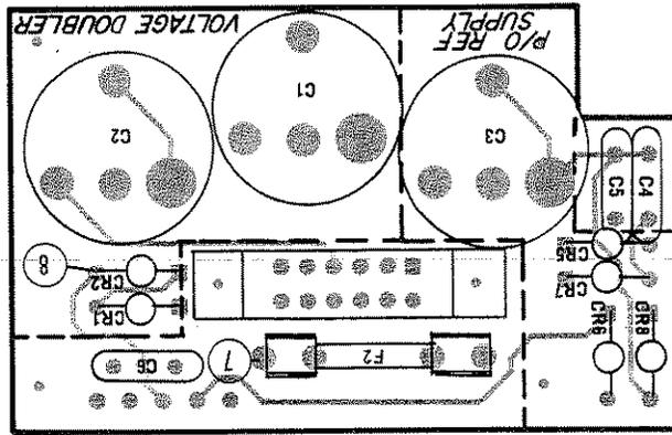
Figure 7-1. A1 Input Board (6177C), Component Locations
