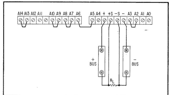
**Figure 3-7. Remote Sensing**
