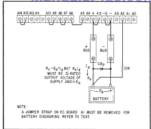
Figure 3-11. Battery Discharging
