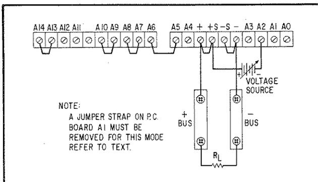
Figure 3-4. Remote Resistance Programming, Constant Voltage, Unity Gain
