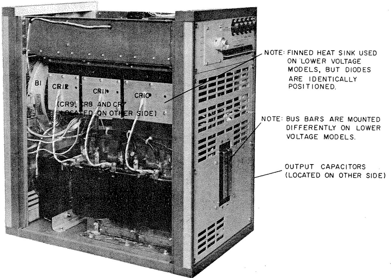
NOTE: FINNED HEAT SINK USED ON LOWER VOLTAGE MODELS, BUT DIODES ARE IDENTICALLY POSITIONED.
