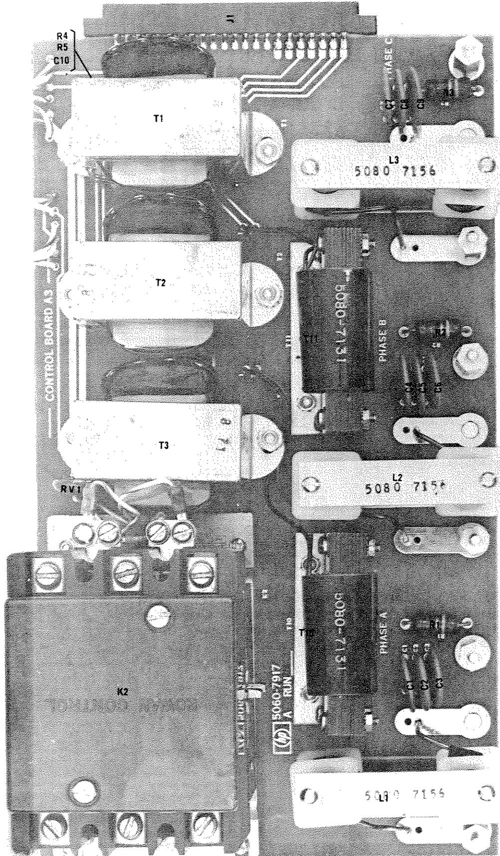
Figure 7-3. A3 Control Board, Component Location
