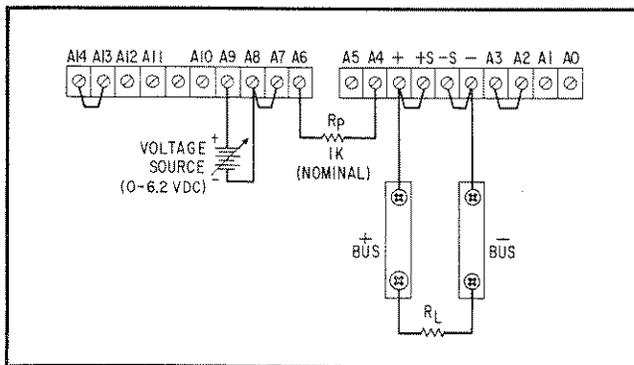
**Figure 3-6. Remote Voltage Programming, Non-Unity Gain, Constant Current**
