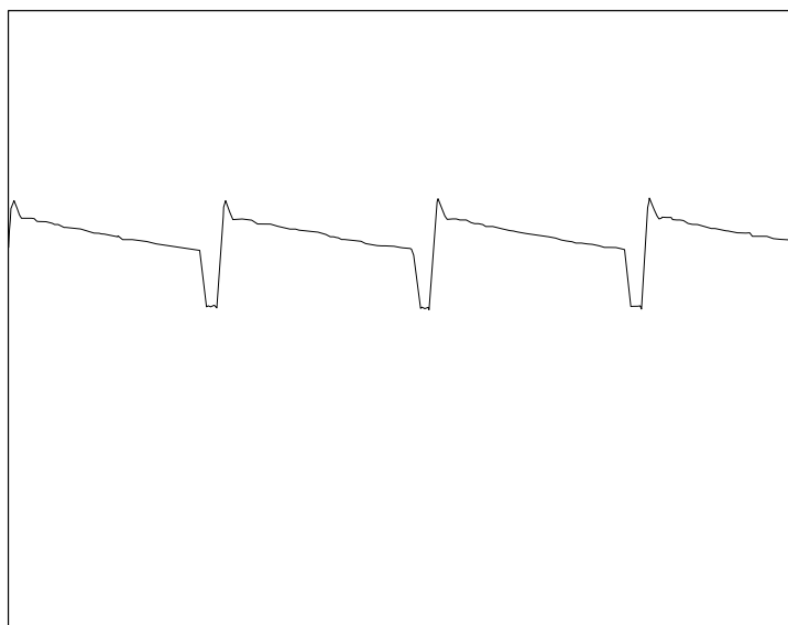
Figure 12-8 Buck Regulator Waveform
