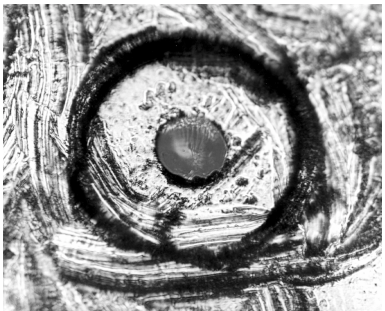
Figure 1-6. Damage from improper cleaning.
