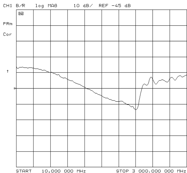
Figure 2-35 Example Mixer LO to RF Isolation Measurement
