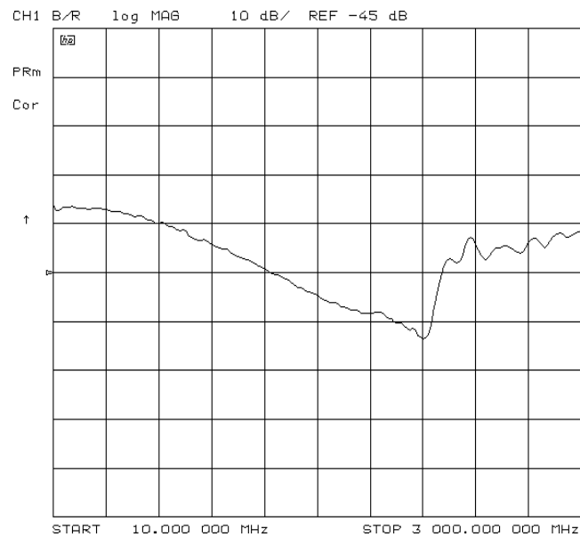
Figure 2-35 Example Mixer LO to RF Isolation Measurement
