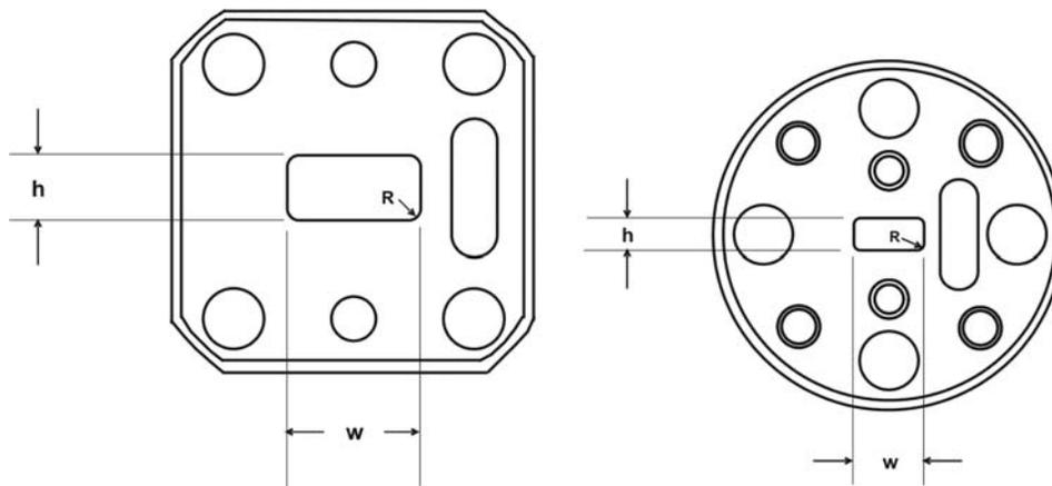
Table 2-2 Mechanical Characteristics of  $\frac{1}{4}$  Wavelength Shims
