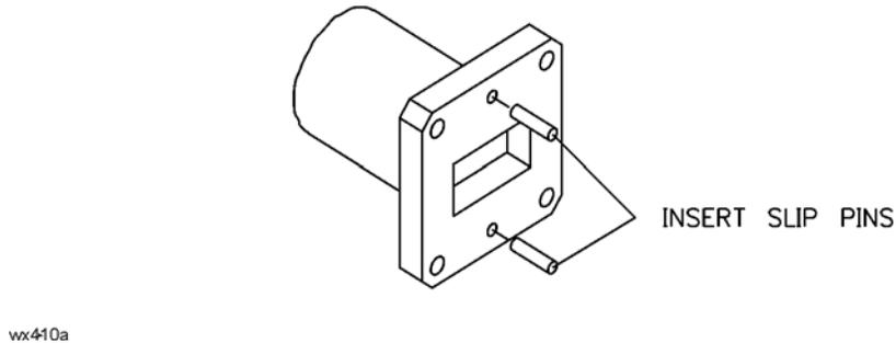
2. Using the pins as guides, carefully align the flanges and insert two screws in the diagonal corner holes, as shown in [Figure 4-4](#).
