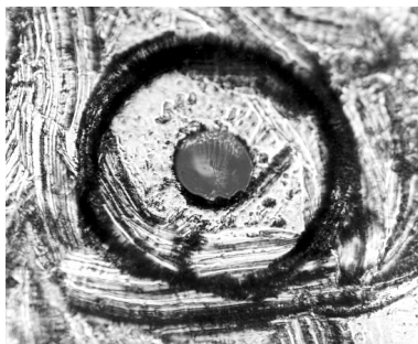
Figure 4-7. Damage from improper cleaning.
