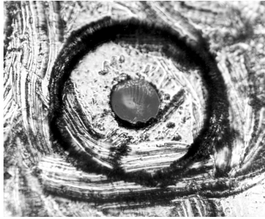
Figure 6-7. Damage from improper cleaning.
