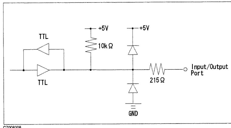
**Figure 8-4. Circuit of Bi-directional Port**
