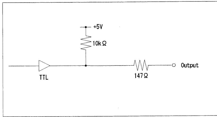
Figure 8-8. Circuit of output
