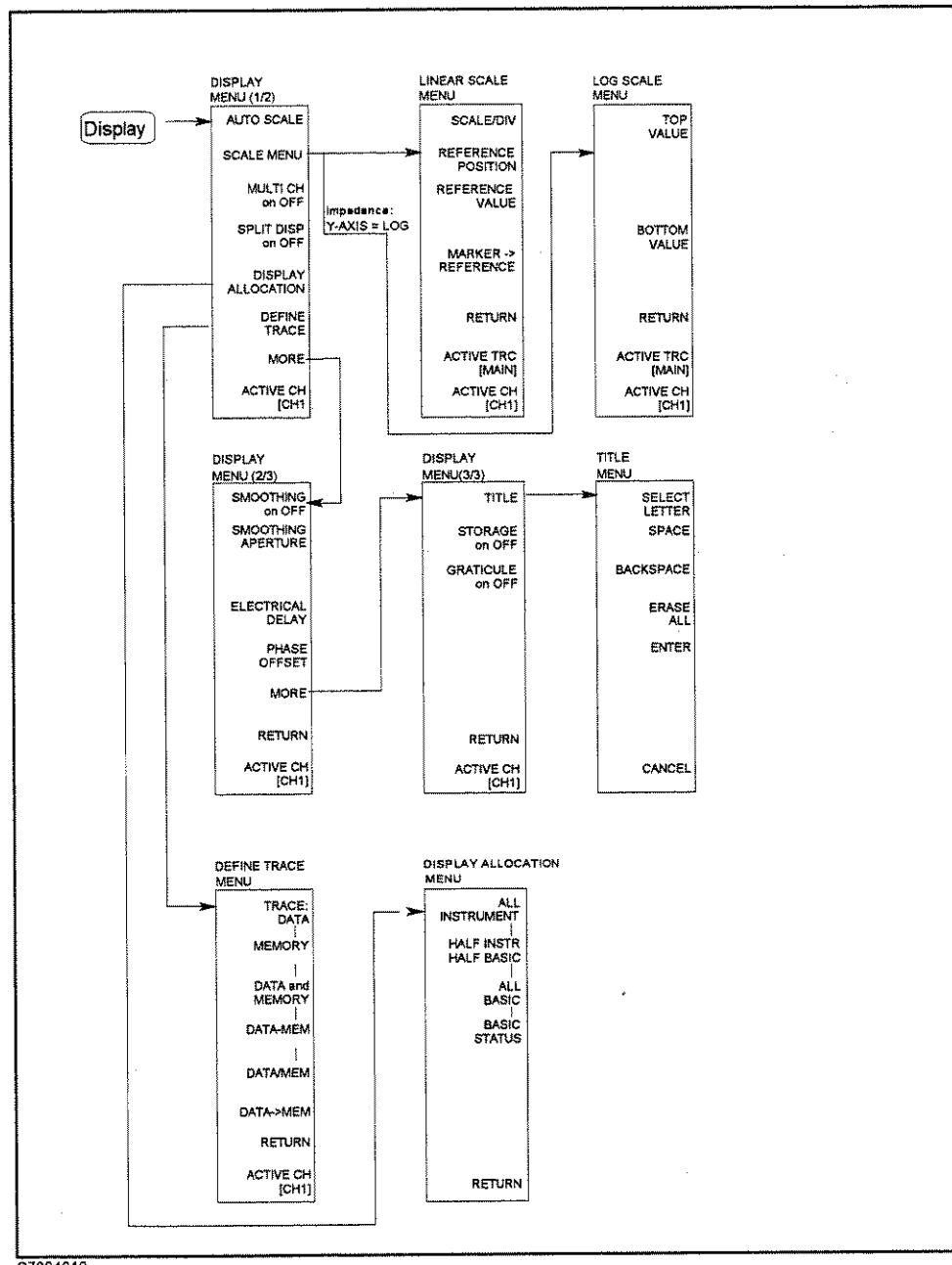
Figure 4-5. Softkey Menus Accessed from the **Display** key
