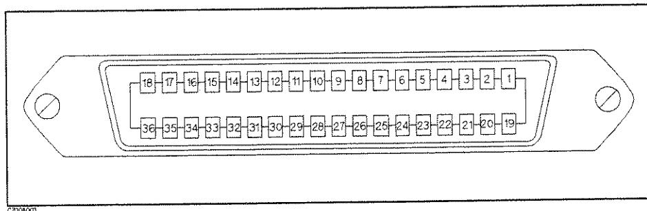
Figure 8-13. Parallel I/O Port Connector Pin Numbers
