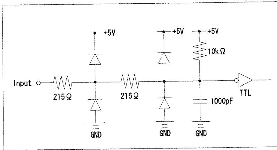
Figure 8-5. Circuit of Input1
