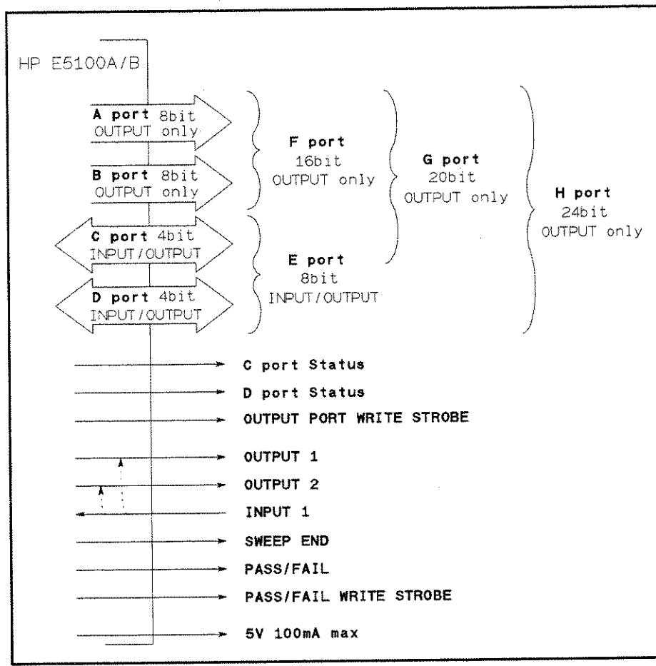
Figure 8-2. Schematic Drawing of Parallel I/O Ports
