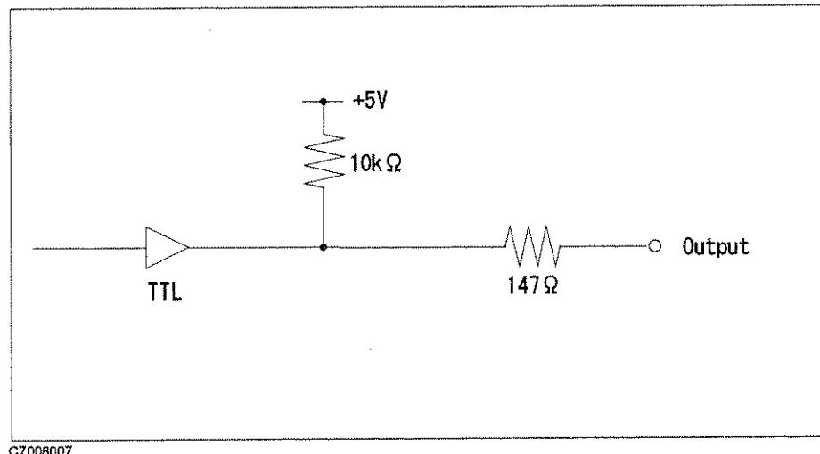
**Figure 8-3. Circuit of Output Port**
