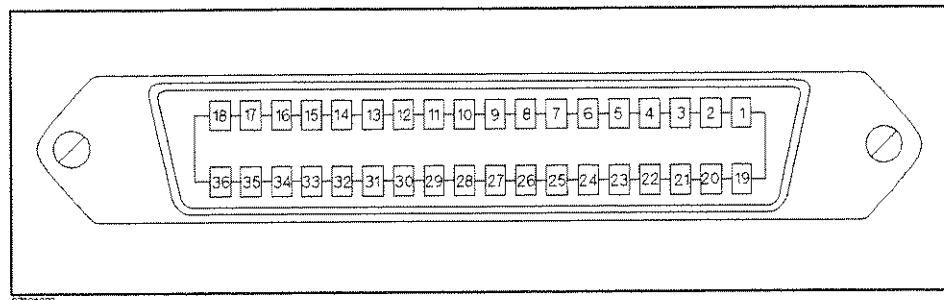
**Figure 8-6. Parallel I/O Port Connector Pin Numbers**
