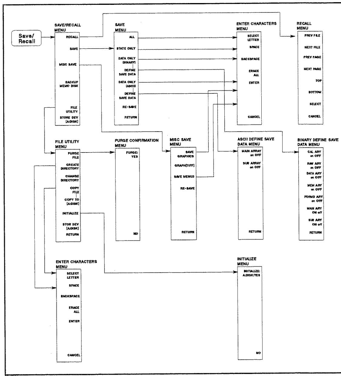
Figure 7-3. Softkey Menus Accessed from the **Save/Recall** Key
