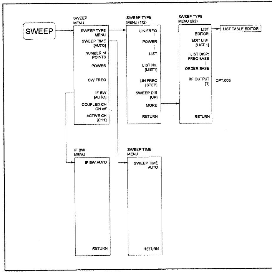
Figure 5-1. Softkey Menus Accessed from the **Sweep** Key
