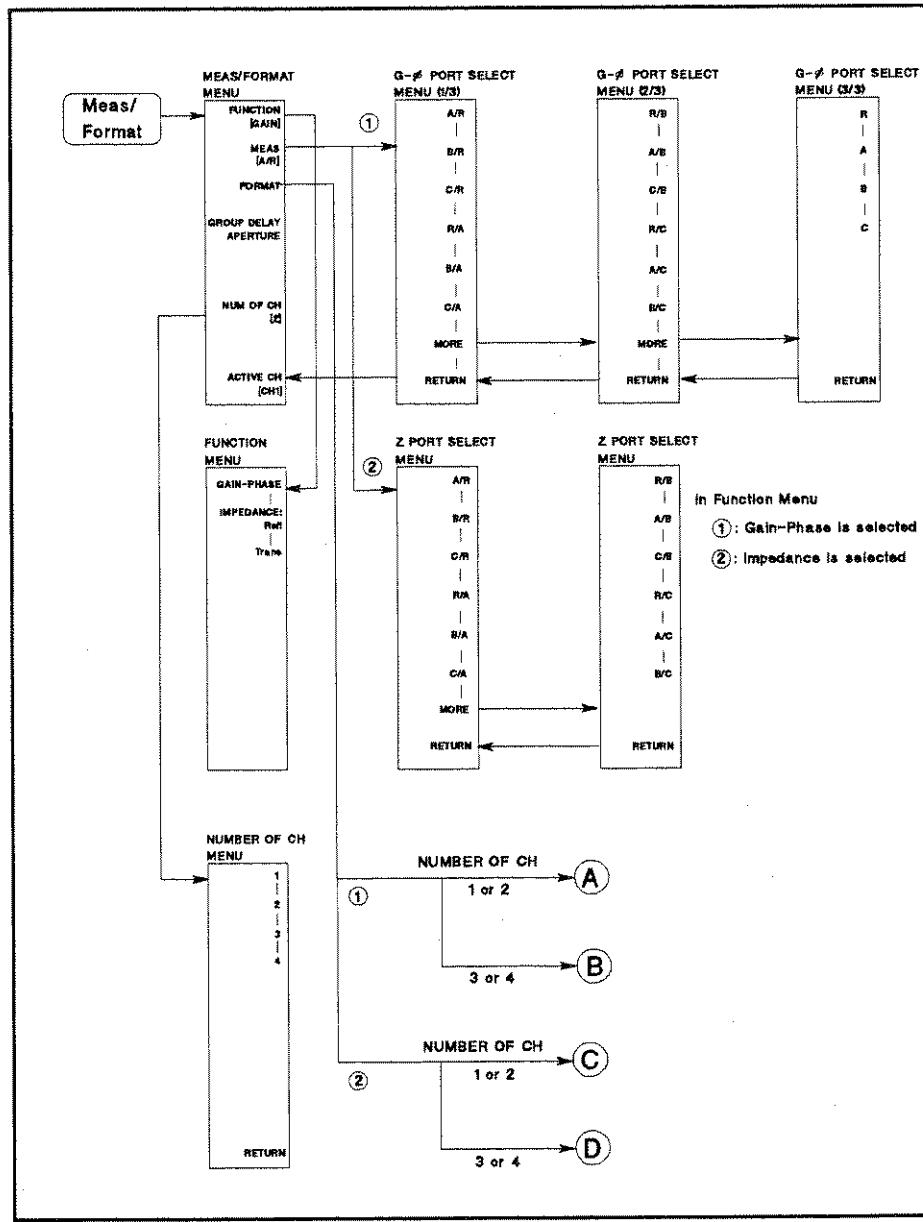
Figure 4-1. Softkey Menus Accessed from the **Meas/Format** Key (1/2)
