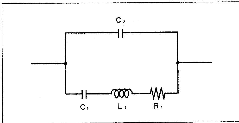
Figure 6-7. Four-Element Equivalent Circuit for Crystal Resonator
