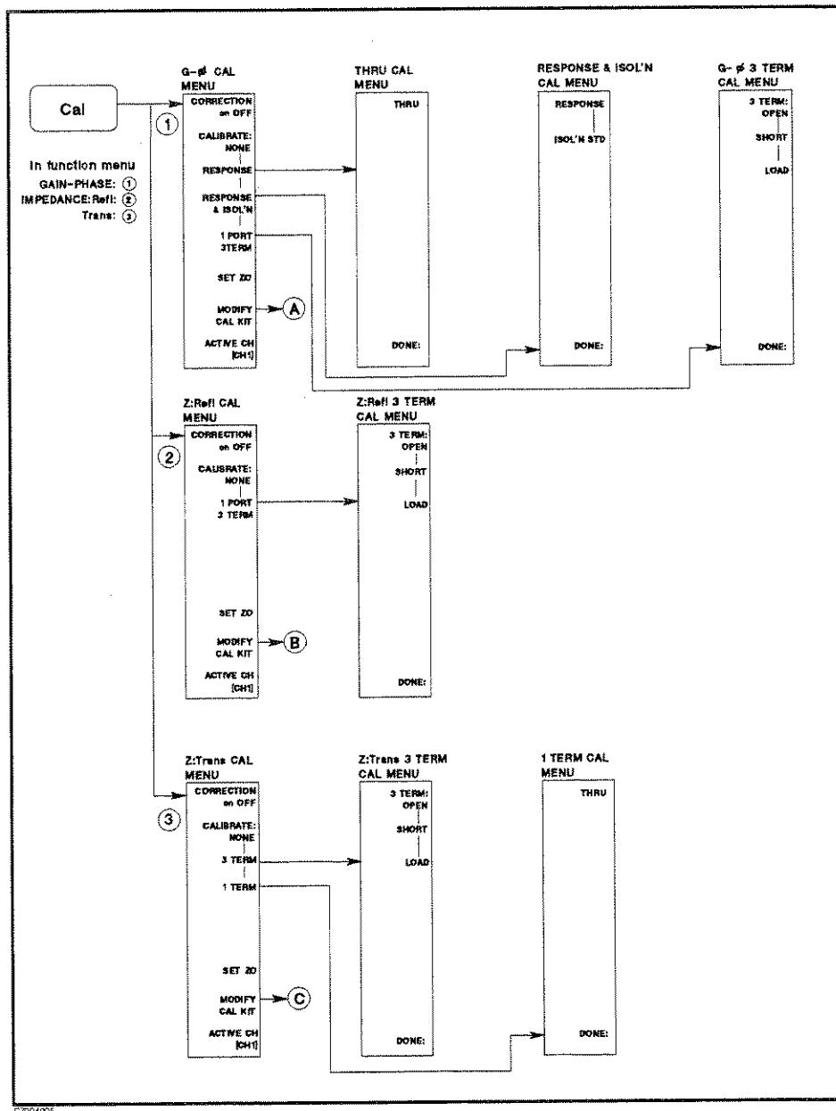
Figure 4-6. Softkey Menus Accessed from the [Cal] Key (1/2)
