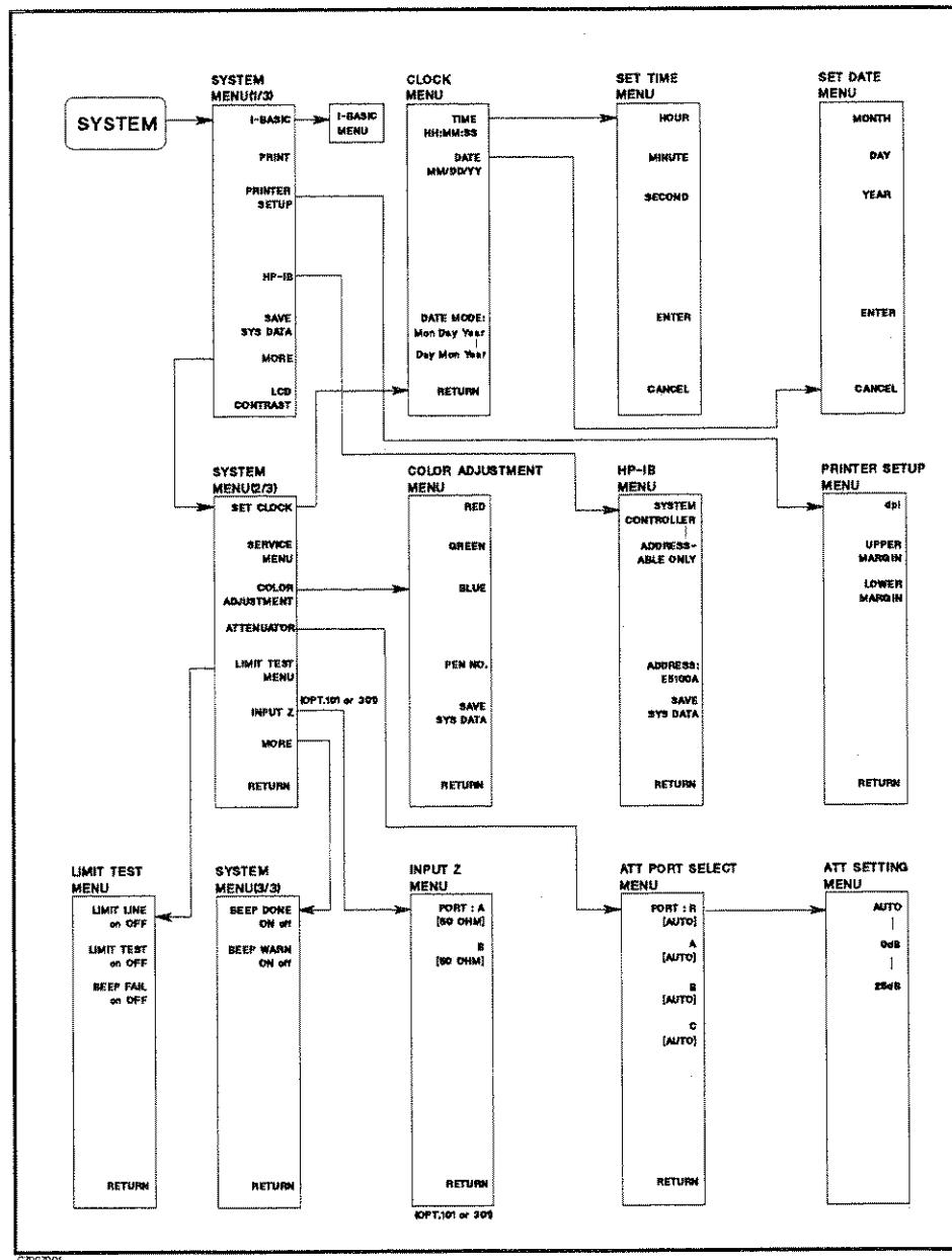
Figure 7-1. Softkey Menus Accessed from the **System** Key
