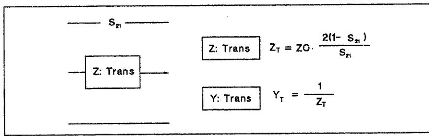
Figure 4-3. Z:Transmission Model
