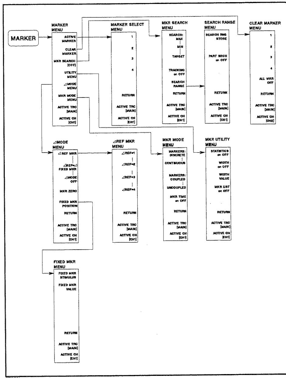
Figure 4-9. Softkey Menus Accessed from the **Marker** key
