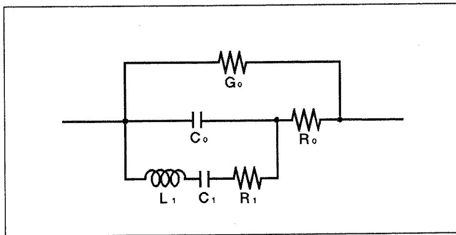
Figure 6-8. Six-Element Equivalent Circuit for Crystal Resonator
