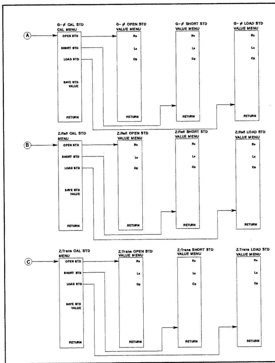
Figure 4-7. Softkey Menus Accessed from the [Cal] Key (2/2)
