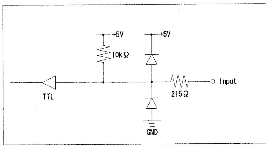
Figure 8-9. Circuit of Input
