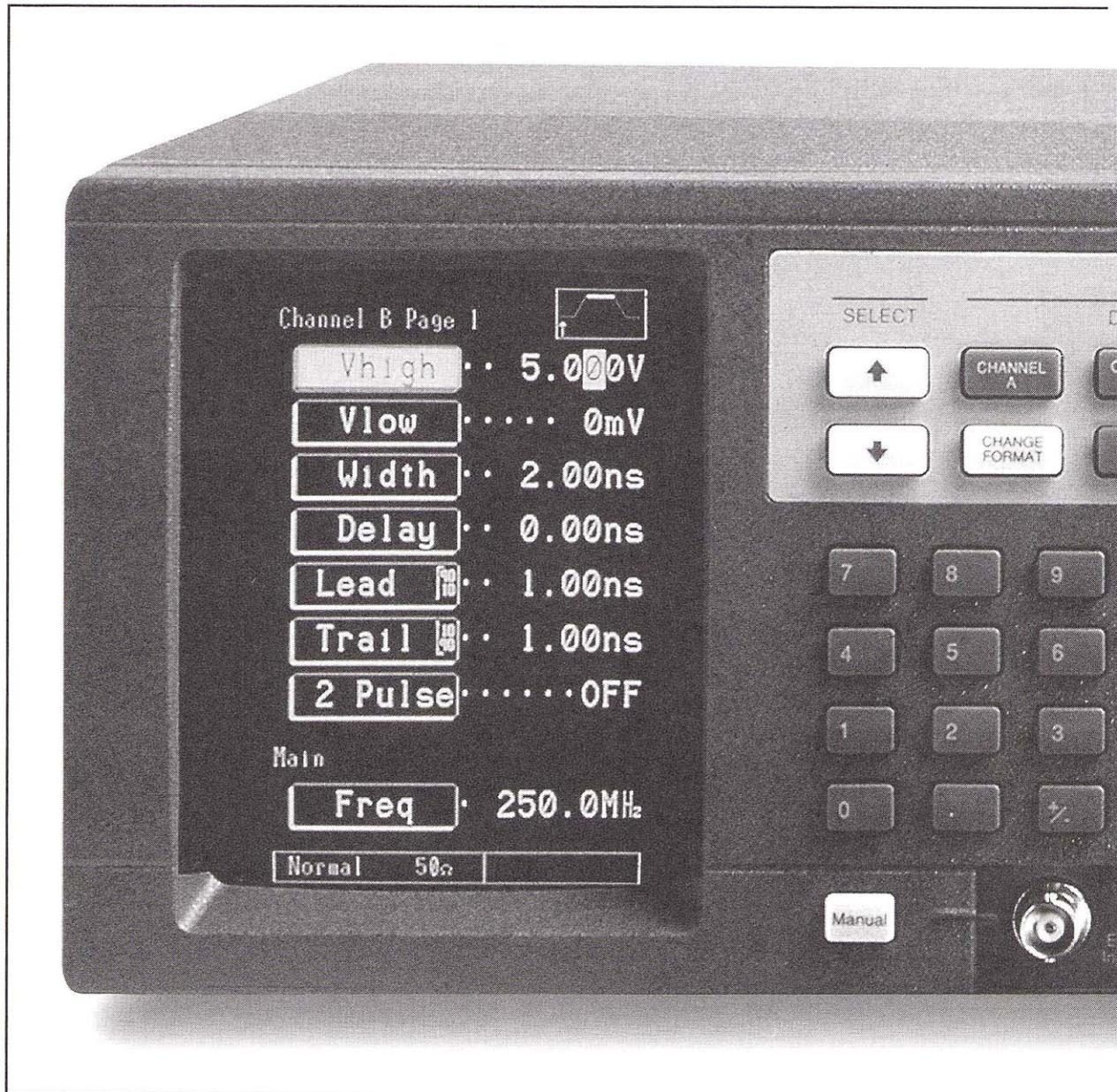
*The 9210 makes it easy to monitor the pulse generator setup. It also changes format to match the way you specify pulses. You can ask for "duty cycle" instead "width" and "frequency" or specify the leading edge risetime in "slew rate" instead of "nanoseconds".*
