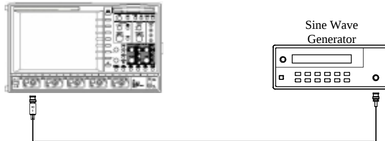
Figure 5-6 : 50Ω Bandwidth Equipment Setup
