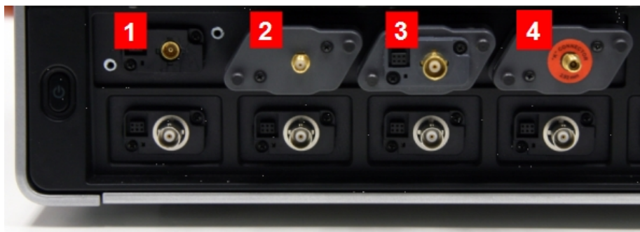
BMA female connector (1). ProLink LPA-SMA, LPA-BNC, and LPA-K-A adapters (2-4).
