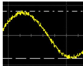
Vertical cursors are lines that you move vertically on the grid to measure the amplitude of a signal.
