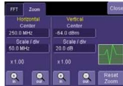
Then use the software zoom controls to change the horizontal and vertical position and scale.
