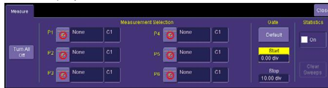
2. The default status is that parameters are OFF, and all are undefined ("None"). Touch either the **icon** or touch in the **None** area to bring up the **Select Measurement** menu:
