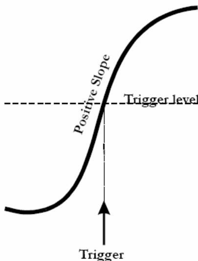
**Trigger Delay** - the amount of time that the oscilloscope trigger is adjusted from a zero value. You can adjust the oscilloscope's trigger position from 0-100% pre-trigger (left to right on the grid), or from 0-10,000 divisions (in time units) of post-trigger.
