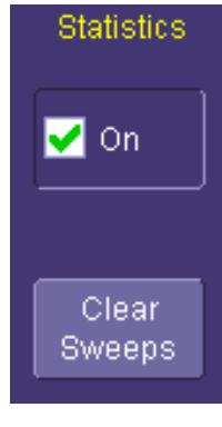
To view measurement statistics, check the box next to **On** under **Statistics** in the **Measure** menu. If a measurement is displayed, statistics will now also be displayed (as shown below).
