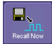
Touch the **Recall Now** button to recall the waveform data file.
