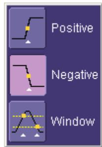
**Positive** and **Negative** slope refer to the direction of voltage change that you want to trigger on.
