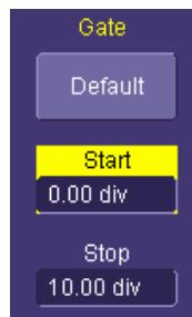
Sometimes you might want to have a parameter measurement on a specific portion of your signal, and ignore all other portions. When this is the case, you can use Measure **Gate**. Measure **Gate** is controlled in the Measure menu, and is set in grid divisions.
