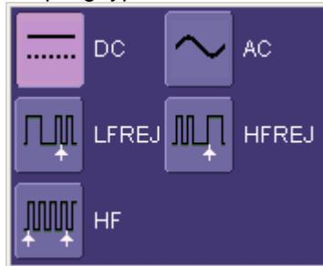
**DC** – All the signal's frequency components are coupled to the trigger circuit for high frequency bursts or where the use of AC coupling would shift the effective trigger level.
