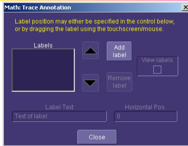
4. Create **Label Text** by using the pop-up keyboard. You may also change **Horizontal Position** of each label, **Remove Label**, and turn labels on/off by checking or unchecking the **View Labels** checkbox.
