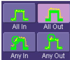
This selection means, for example, that if you select **All In** the test will be False if even a single waveform falls outside the mask.
