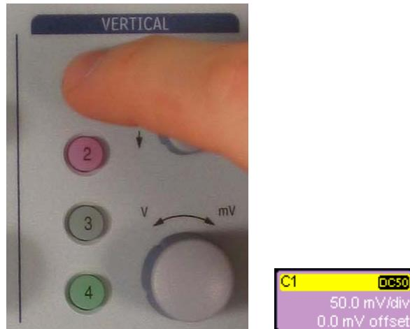
3. If the signal is not on the grid, press the **AUTO** trigger button and adjust **Horizontal** and **Vertical** front panel
