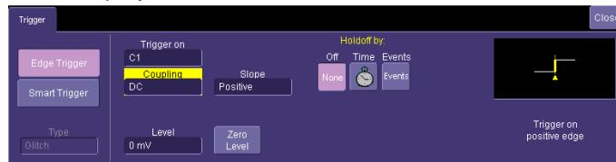
Make sure that **“Edge Trigger”** is highlighted, and not **“SMART Trigger”**
