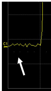
The Zero Level Indicator is a color-coded label that is positioned vertically on the grid.
