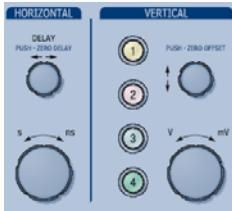
Then use the front panel horizontal and vertical controls to adjust position and scale. The operation of the knobs will feel natural. Use the table below as a guide.
