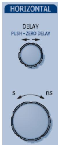
Set up the timebase by using the front panel **Horizontal** controls, just as for analog scopes. The WaveSurfer will allocate memory as needed to maintain the highest sample rate possible for the timebase setting.
