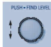
To change Trigger Level, use the front panel knob in the Trigger Control area. Rotate knob to adjust, or push to set to 50% of the signal level.
