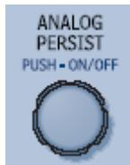
The analog Persistence feature helps you display your waveform and reveal its idiosyncrasies or anomalies for a repetitive signal. Use Persistence to accumulate on-screen points from many acquisitions to see your signal change over time. Press the knob to turn persistence ON to "Analog" mode, press again to view "Color-graded" mode, and press again to turn OFF. Rotate the knob to adjust the saturation of the persisted waveforms.
