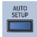
Automatically sets timebase, trigger, and sensitivity to display a wide range of repetitive signals.
