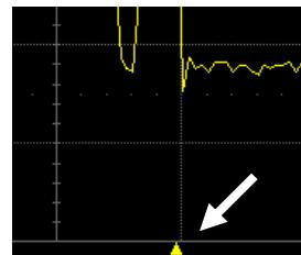
The Trigger Delay Indicator is a color-coded triangle that is positioned horizontally on the grid.
