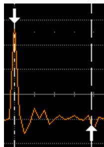
**Horizontal (Frequency)** cursors are moved horizontally along the FFT Math trace. Place them at a desired location along the frequency axis to read the signal's frequency and amplitude at the selected location.
