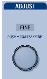
To set the gate, touch the **Start** field to highlight the control yellow, and then use the adjust knob to adjust the location of the start gate. Repeat for the **Stop** gate. Measure gates will remain on the display as long as the **Start** gate is not equal to 0 divisions, and the **Stop** gate is not equal to 10 divisions.
