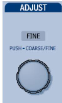
The adjust knob can be used to make adjustments to a value when a menu is open and the selected control has a yellow highlight.
