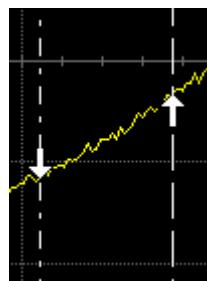
Horizontal (Time) cursors are moved horizontally along the waveform. Place them at a desired location along the time axis to read the signal's time and amplitude information at the selected location
