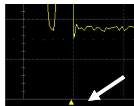
The Trigger Delay Indicator is a color-coded triangle that is positioned horizontally on the grid.
