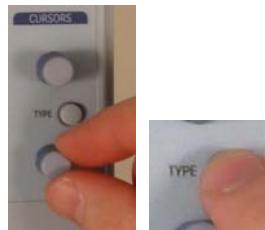
Cursors will automatically turn on when you rotate either of the two cursor knobs. Or, you can press the **Type** button to turn cursors ON, then toggle through the various cursor types.
