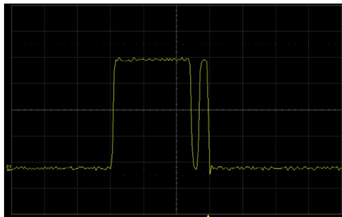
The grid area is divided into 8 vertical divisions and 10 horizontal divisions, just like any other oscilloscope. There are several indicators on the grid to help you understand the following:
