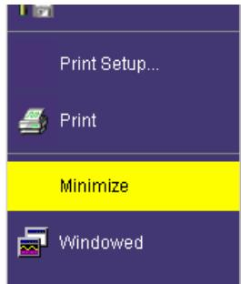
You can access the WaveSurfer's (Windows) desktop by opening the **File** Top Menu Bar and then choosing **Minimize**. This will minimize the oscilloscope and allow you to open other Windows programs, such as Windows Explorer, Paint, Internet Explorer, etc.
