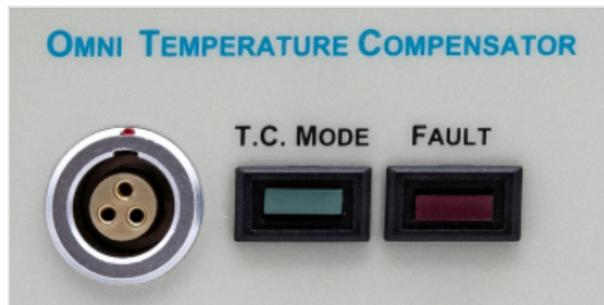
The TCM feature of the 4176, arithmetically calculates the resistance value to display utilizing the ambient temperature and other parameters that will be present in later chapters. It is solemn for the user to be aware if the TCM mode is enabled or disabled so that the display reading may be interpreted correctly.
