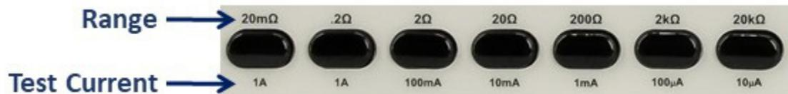
Ranges are easily selected by pressing the appropriate key. The range keys are labeled using the value of the range and the respective test current value. The range selected will be displayed on the range window. To return to the auto range mode, press the "AUTORNG" key on the front panel.
