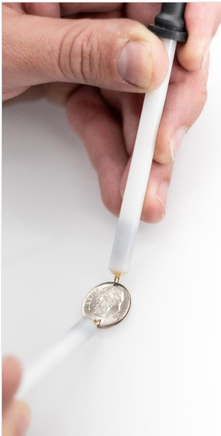
For flat surfaces, you can choose between two different spring-loaded surface probes. If this is your choice of leads, simply press one probe against one side of the surface of your load, making sure that the surface of the probe is in full contact with the surface of the load. Press the second probe against the surface at the opposite side of your load making sure that the surface of the probe is in full contact with the surface of the load.
