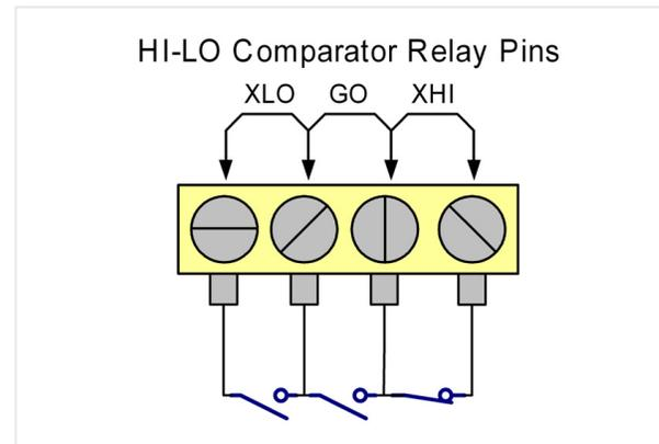
Contacts are rated at 100 volts, 100mA. The truth table of the contacts is listed below. The  $\Omega$ 's symbol represents the load measured value; UL is the upper limit and LL is the lower limit set by the user.
