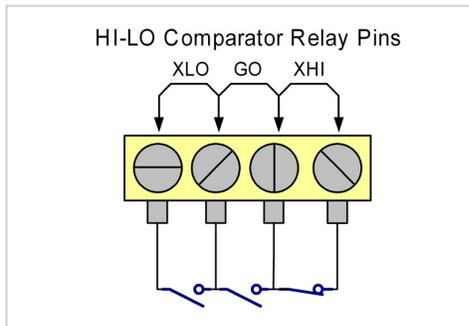
The HLC relay terminal is internally wired to three relays which are active only when the HLC mode is selected. According to the result of the comparison, one of the relays will have its contacts closed while the remaining two relays will have contacts open. The standard "relay contact closure" feature allows an automated sorting process to be set up at an
