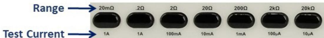
**CAUTION** - Extra care must be taken when working with inductive loads. Always select the highest resistance range before connecting or disconnecting the test leads.
