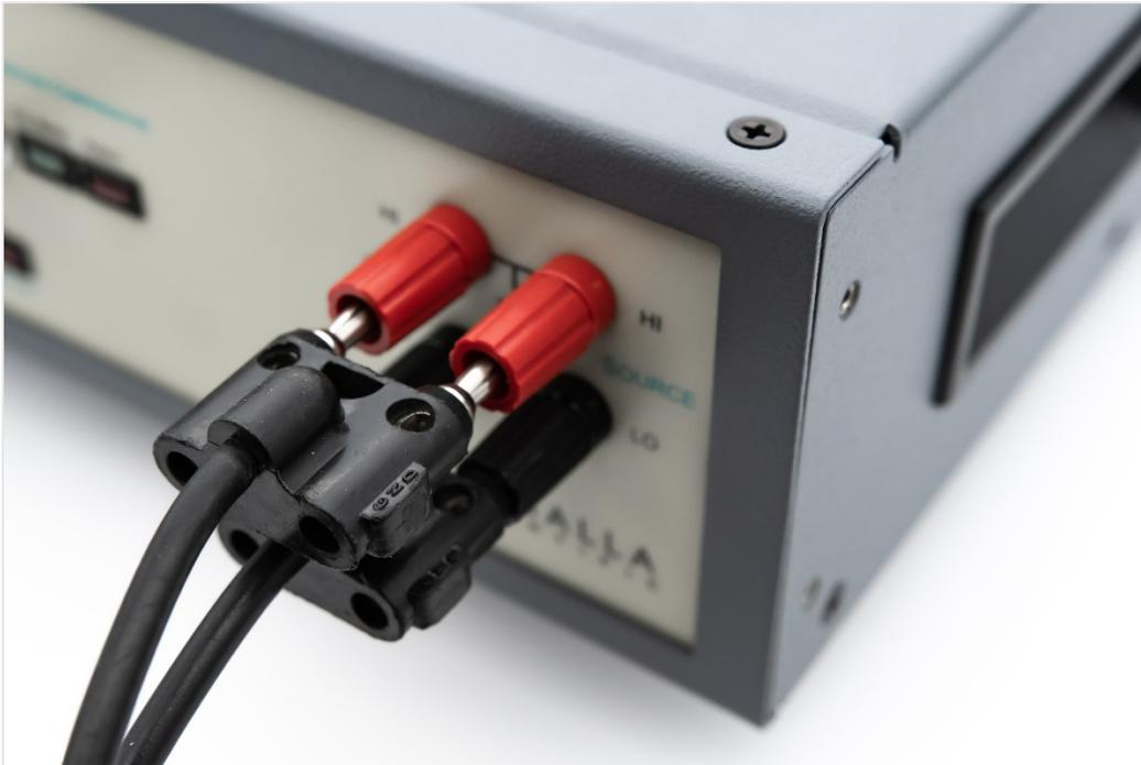
Lead 1 - Connect between SENSE HI and SOURCE HI, with the ground marker on the source side.
