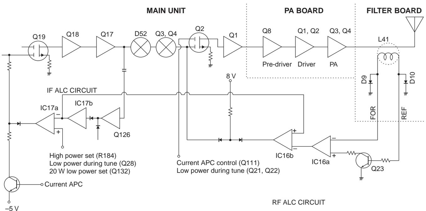
The reference voltage for the comparator is set by R184. The antenna tuning control voltage (TUN8) is also affected by the reference voltage to decrease the IF signal level.
