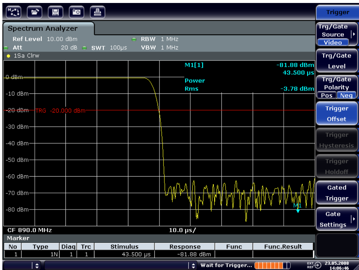
Fig. 2-17: Falling edge of the GSM burst displayed with high time resolution
