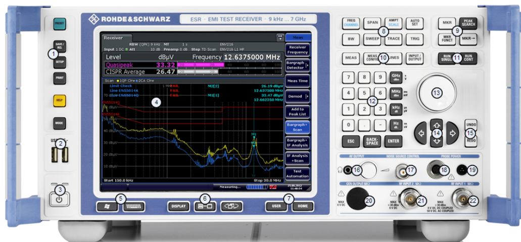
Fig. 2-1: Front panel of the R&S ESR
