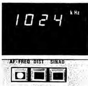
Front-panel section: right-hand display/keyboard for modulation frequency and distortion measurements
