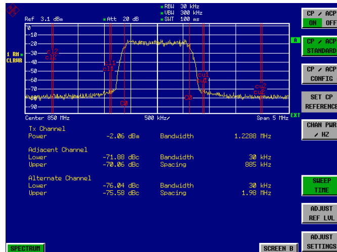
Fig. 2-1 Adjacent channel power measurement on a CDMA IS95 signal
