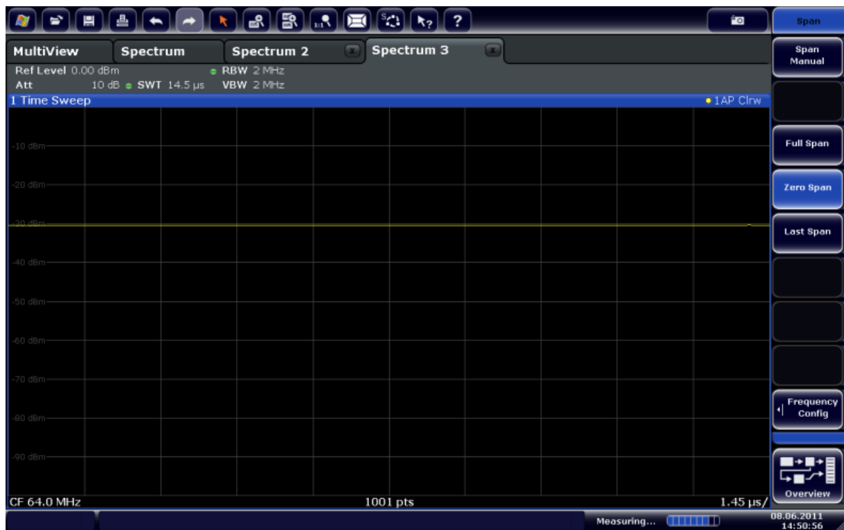
Fig. 4-7: Time domain display of the calibration signal
