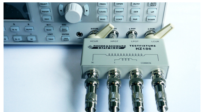
Fig. 8.6: Connecting the measurement adapter to the LCR bridge
