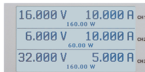
Fig. 4.3: Adjustable maximum values R&S®HMP4030
