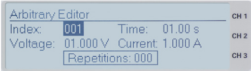
Fig. 5.5: Arbitrary settings (R&S®HMP2030)
