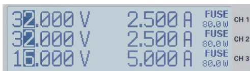
Fig. 5.1: 1-V position for all three channels (R&S®HMP2030)
