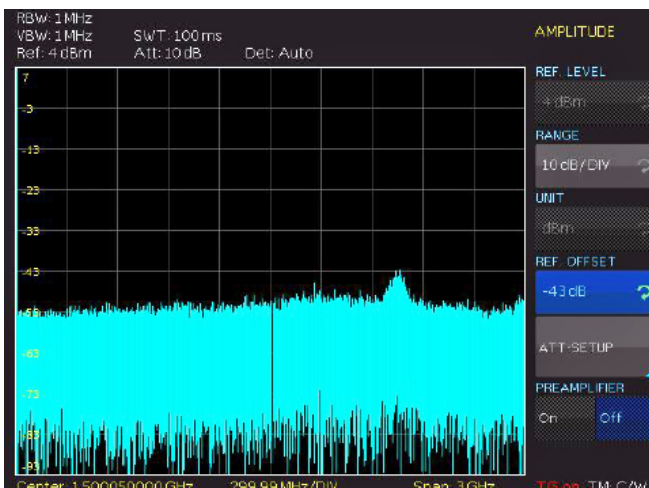
Fig. 6.12: Trace shifting with reference offset
