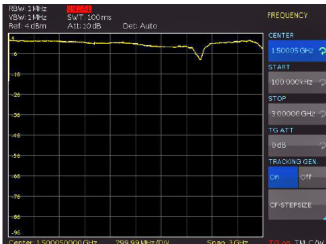
Fig. 6.7: Tracking generator measurement unaligned
