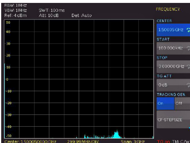
Fig. 6.11: Loosening of the RF cable completely
