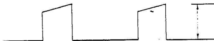
Fig. 5-1 Primary voltage characteristics of the DC-DC converter
