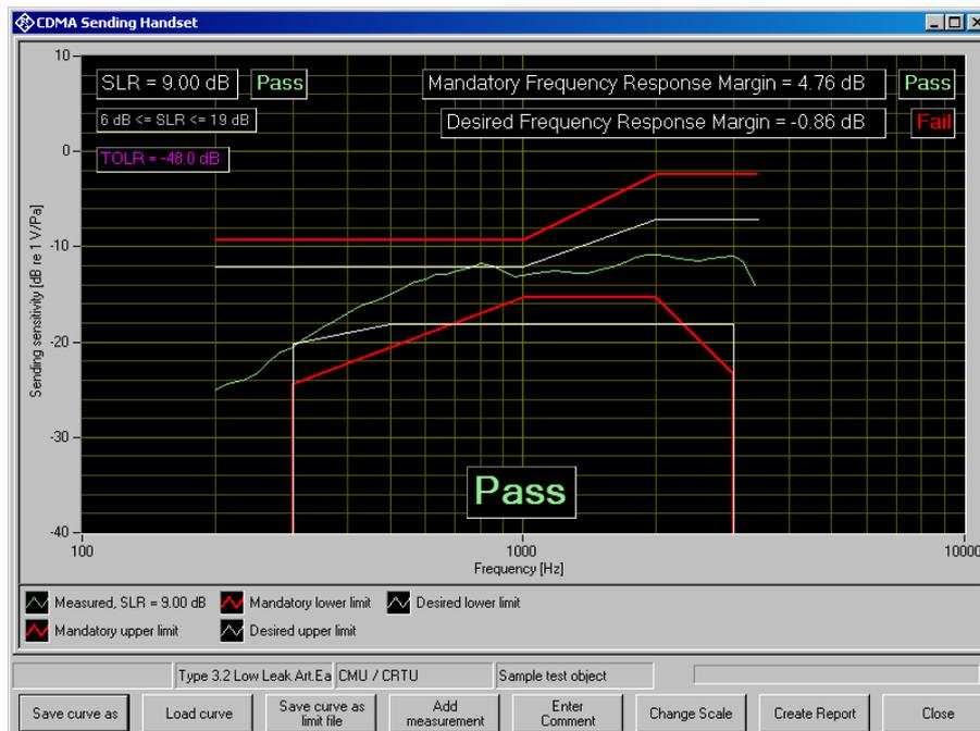
Figure 6-6: Sending frequency response with SLR value displayed
