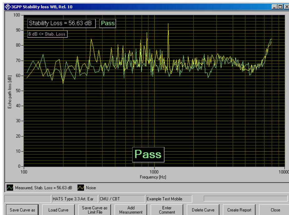
Figure 6-13: Window of stability loss test
