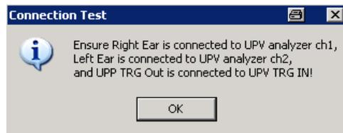
Figure 4-31: Instructions for change of cabling during the calibration process
