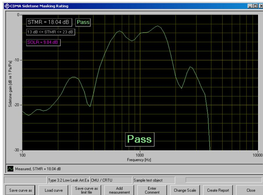
Figure 6-10: Typical Measurement of sidetone masking rating
