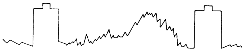
Figure 4 Normal Video and Sync Signal.
