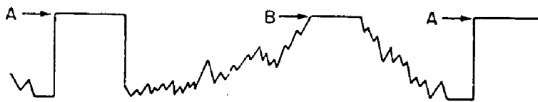
Figure 5—Overloaded or Clipped Video and Sync Signal.
