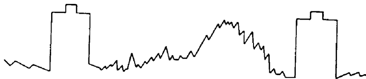
Figure 4—Normal Video and Sync Signal.
