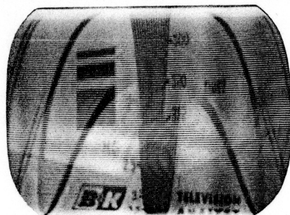
Figure 14—Sweep developed using vertical yoke test signal
