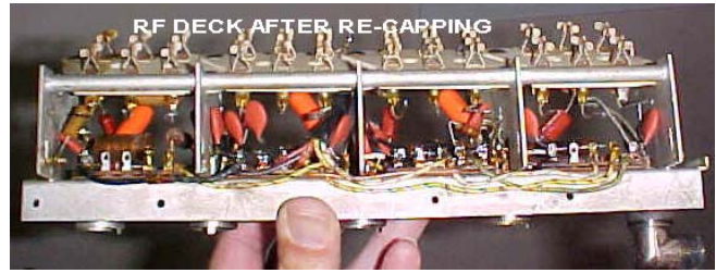
RF Deck after
