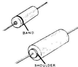
NOTE: When installing the tubular capacitors, be sure that the end marked with a band or shoulder is placed as shown in Pictorial 2.
