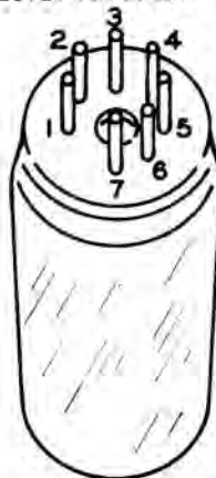
BOTTOM VIEW OF TUBE SHOWS CLOCKWISE PIN NUMBERING STARTING AT WIDE SPACE BETWEEN 1 AND 7.
