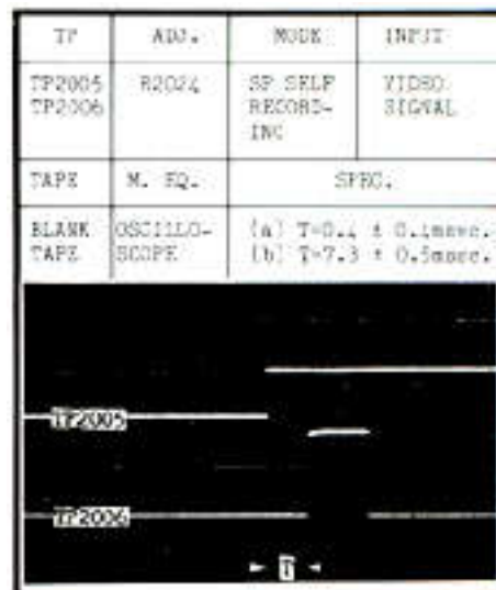
Fig. 8: Tracking fix adjustments usually require that you adjust a signal for the correct delay from the head-switching square wave.
