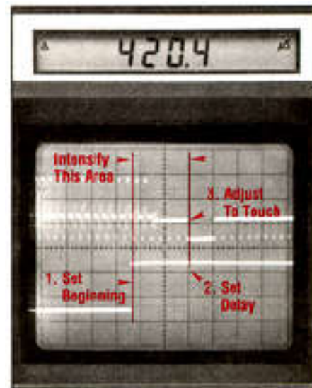
Fig. 7: Use the Delta Time function to pre-set the time needed between signals, and then adjust the circuits until the signals touch the intensified area of the waveform.
