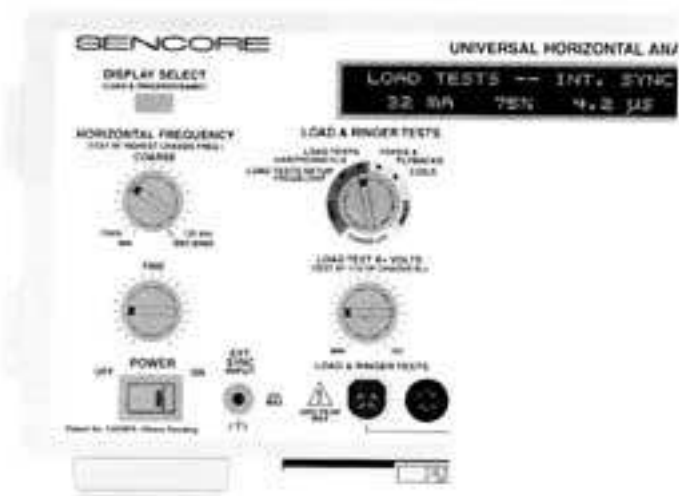
Fig. 5: The Load Tests indicate if the horizontal output stage contains a defect.
