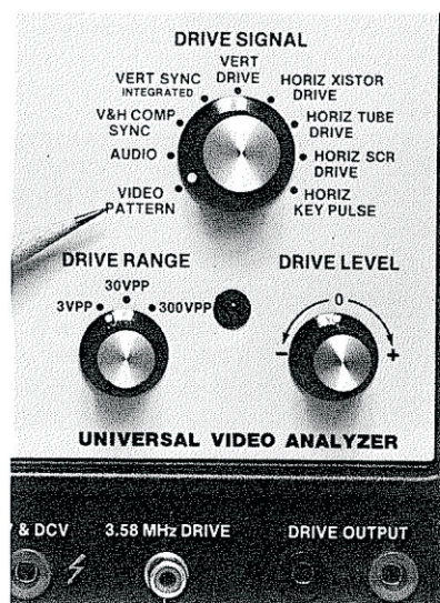
Fig. 30 — The DRIVE SIGNAL switch selects the correct signal to inject into any stage after the detectors. The output level is controlled by the DRIVE RANGE switch and the DRIVE LEVEL control and supplied through the isolated DRIVE OUTPUT jacks.
