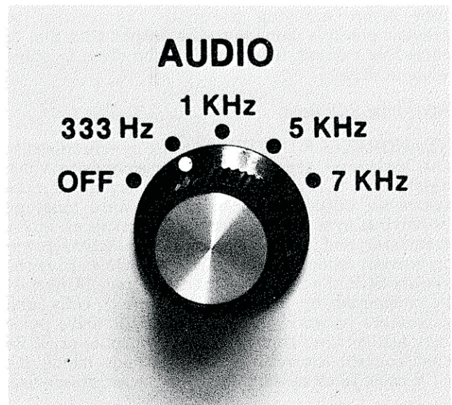
Fig. 36 — The AUDIO switch selects one of four audio tones to modulate the RF and IF signals, or to feed to the DRIVE SIGNAL "Audio" function.
