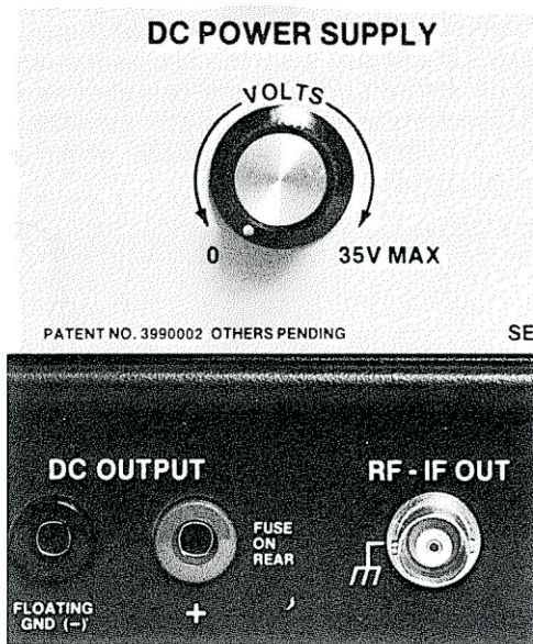
Fig. 27 — The DC POWER SUPPLY provides an adjustable, regulated DC voltage. The outputs are floating to allow connection to non-grounded circuits.
